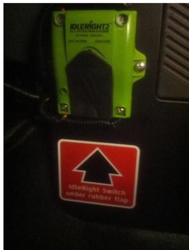
The IdleRight2 will eliminate the need to idle for the purposes of police operational needs. The patrol officer will be able to run all electronic accessories while the engine is off without fear of running down the vehicle battery.
