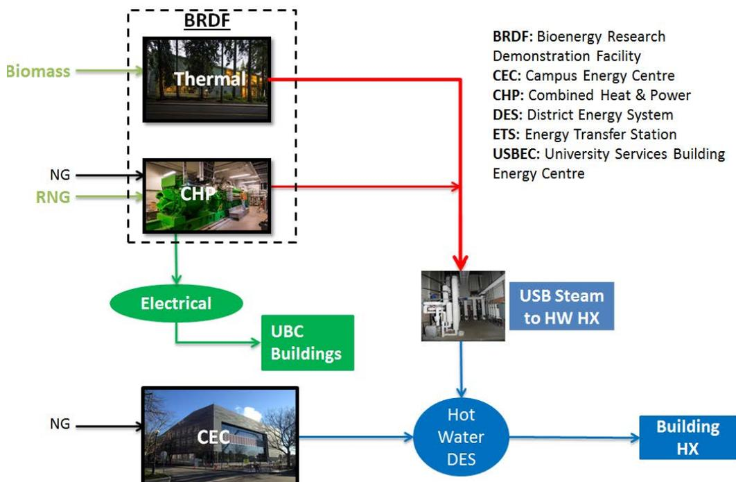
Figure 1 – UBC Thermal & Electrical Generation
