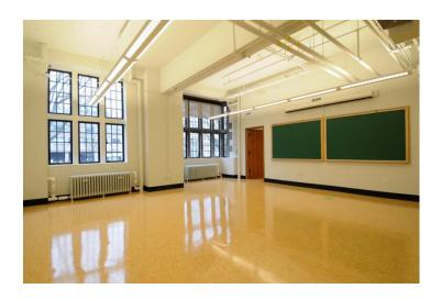
Cross-ventilation delivers fresh air and free cooling without fans, and the building's highmass stone and concrete elements maintain relatively stable indoor comfort conditions, absorbing "cool" from the prevalent summer breezes, and solar radiation from the low winter sun.
