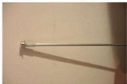
above right: steel rod with bent cable strap fittings creating hinge, poly tubing spacer allows for non-horizontal edges
