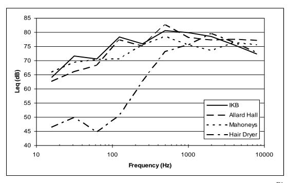
Figure 1: Measured variation with frequency of the average noise levels (Leq) of the Dyson Airblade<sup>™</sup> hand dryer taken in Irving K. Barber (IKB), Allard Hall, and Mahoney & Sons, and from a typical hair dryer.
