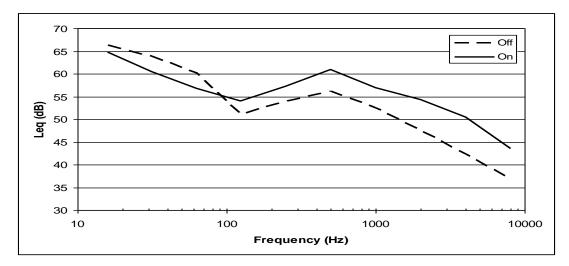
Figure 2: The variation with frequency of average noise levels (Leq) measured in the occupied hallway outside the IKB washroom, when the Dyson Airblade<sup>™</sup> hand dryer was on and off.
