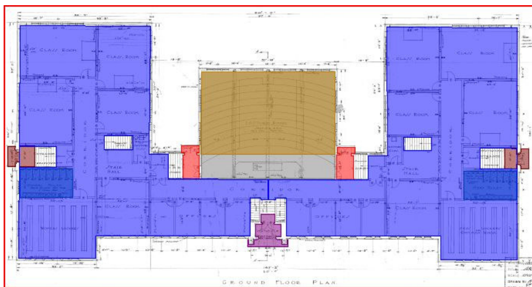
Figure 3 - OST screenshot showing area takeoffs for floors on the ground floor of the Math building
