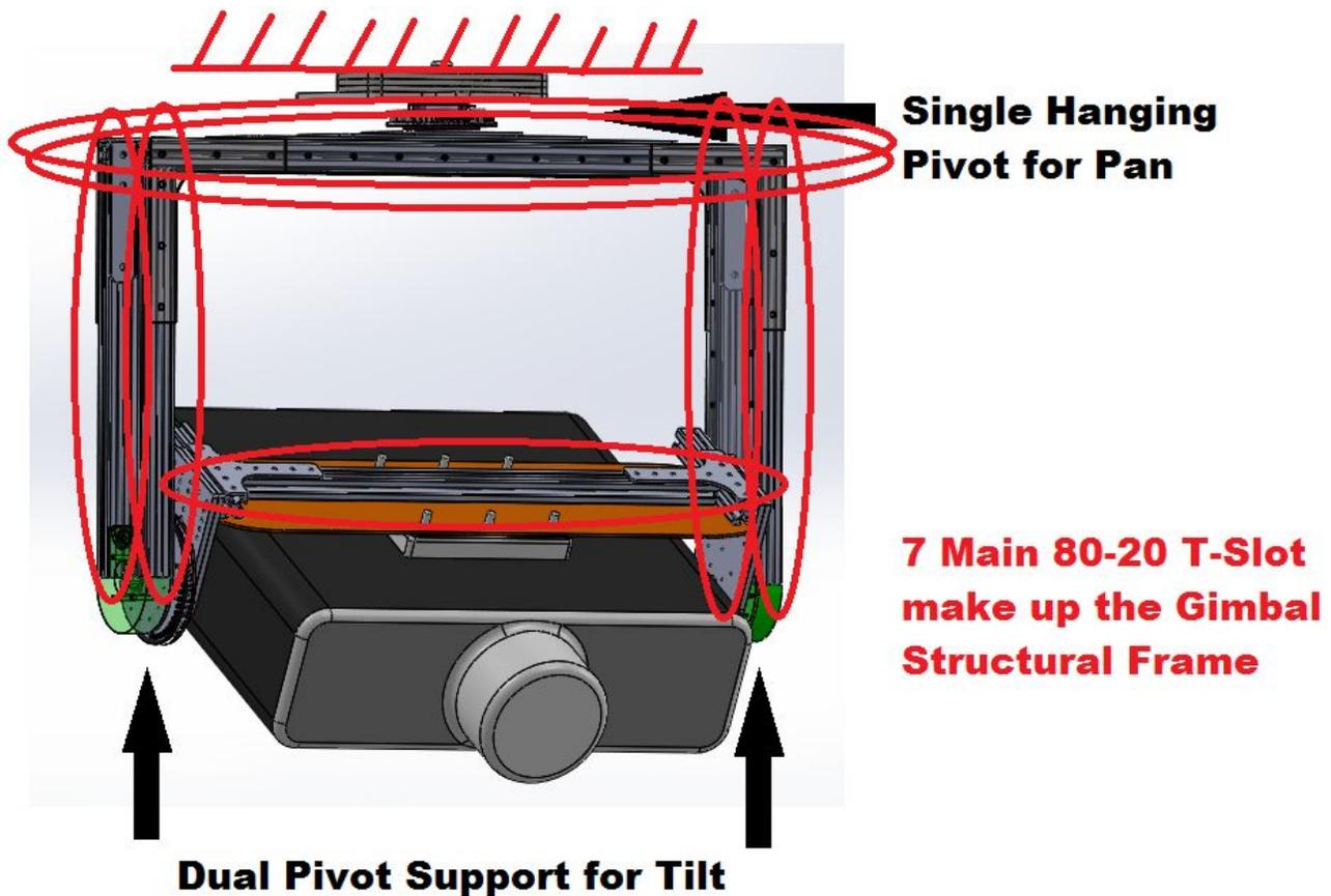
*Figure 2.1 - Gimbal Style Structural Frame*
