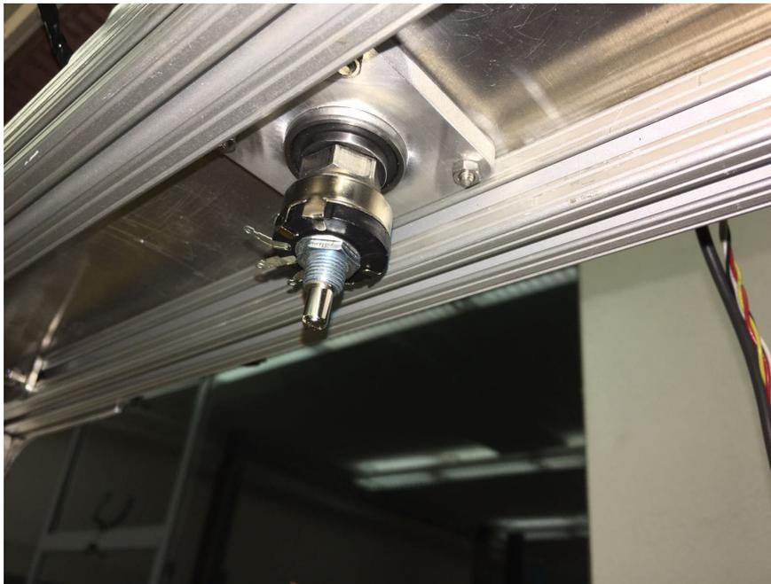
*Figure 3.1 Position of potentiometer*
