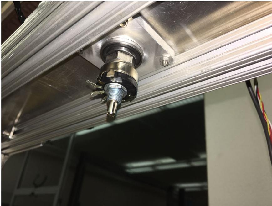
*Figure 3.1 Position of potentiometer*
