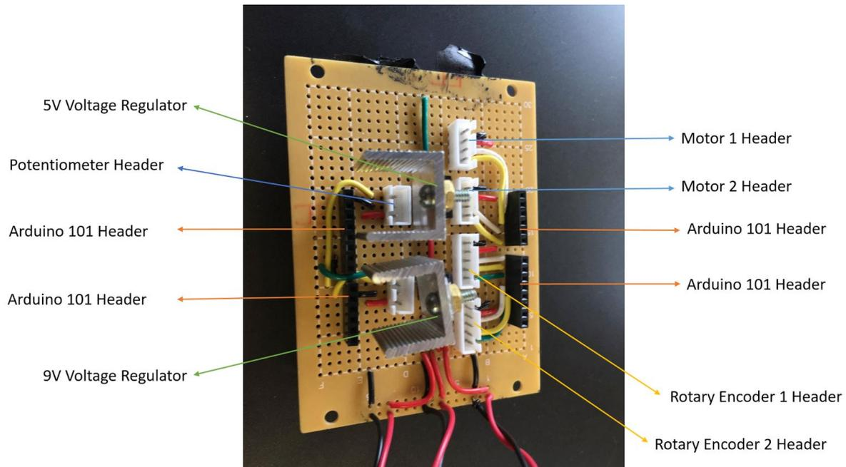
*Figure 6.4- Protoboard Circuit Diagram*
