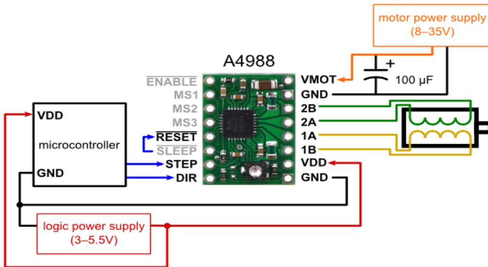
Figure 6.1: Circuit Diagram of the motor driver
