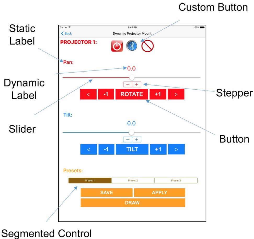
*Figure 4.2 - Projector 1 View with User Interface Elements Identified*
