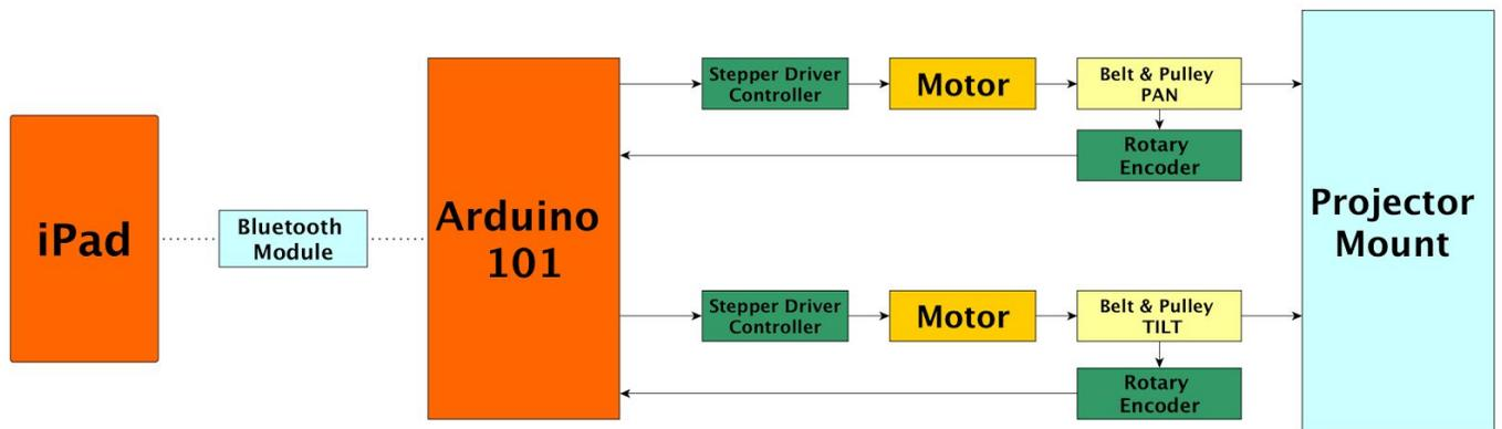
Figure 1.1 - System Block Diagram Project Overview
