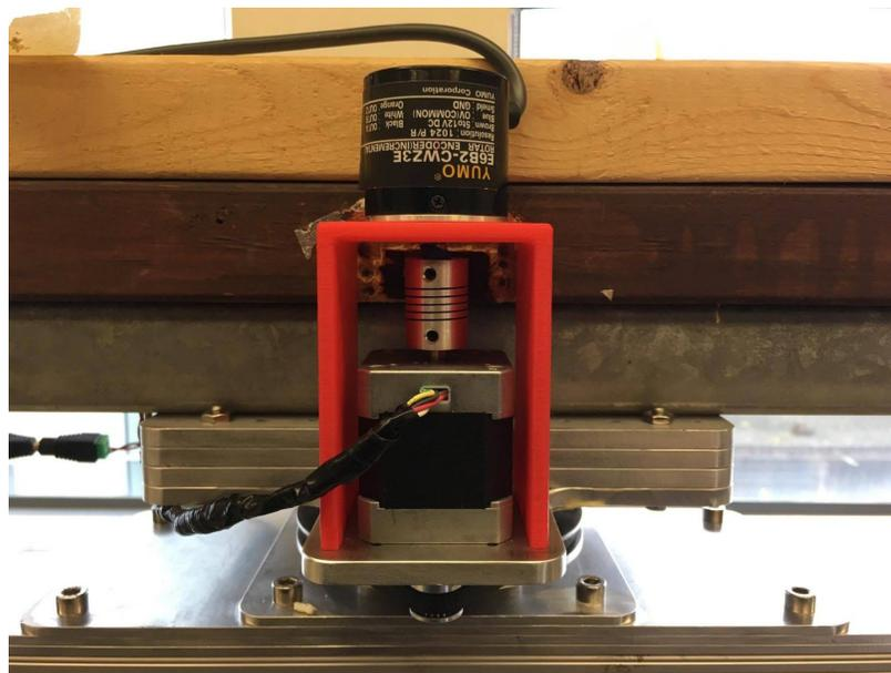
Figure 3.2 Motor Coupled with the Rotary Encoder
