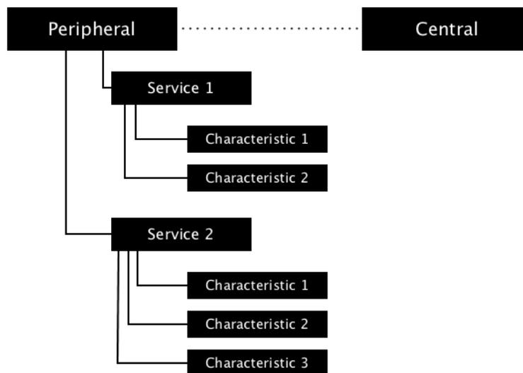
*Figure 4.1 Block Diagram of an Example Peripheral & Central*
