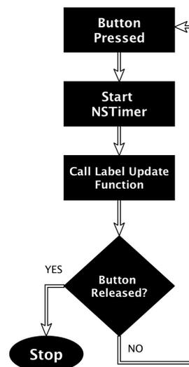
Figure 4.4 - Real-Time Movement Block Diagram
