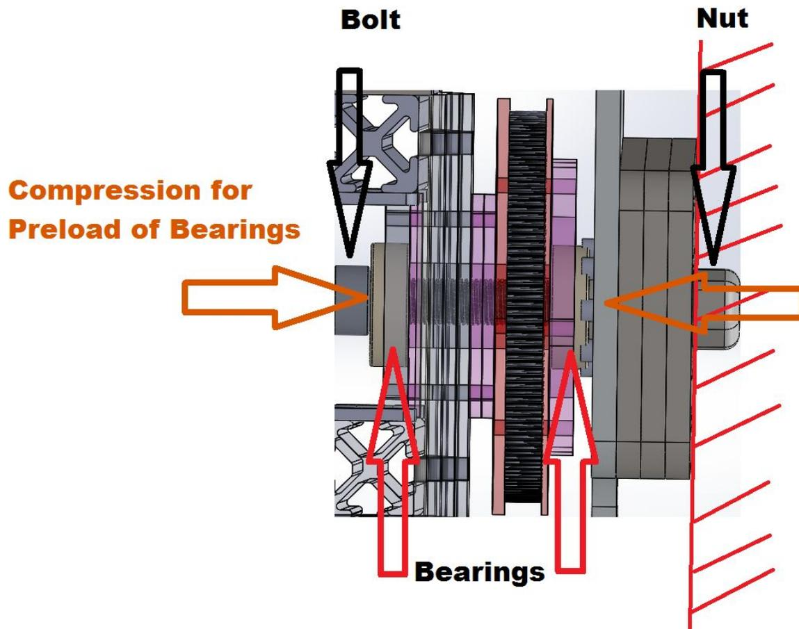
*Figure 2.2 - Pan Dual Bearing Compression Preload*
