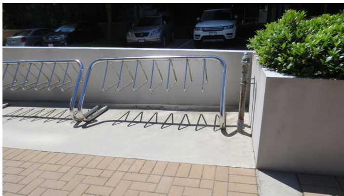
Figure 29: At Sage, cluster racks are not ideal as they force bicycles together and fit only standard bicycles. If necessary, they could be used for Class II storage only.
