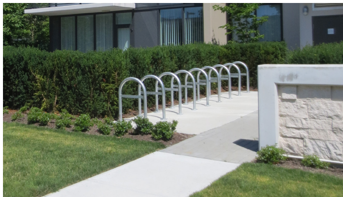
Figure 30: At the Laureates, inverted U or staple racks are simple and efficient. A low bar can provide small bicycles something to lean against.
