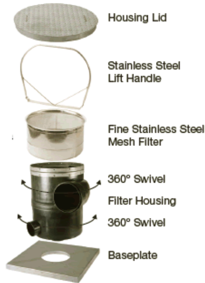
Figure 15: In-line Filter Connection
