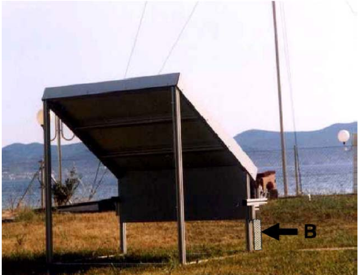
Figure 3: Dew condenser system used in Croatia
