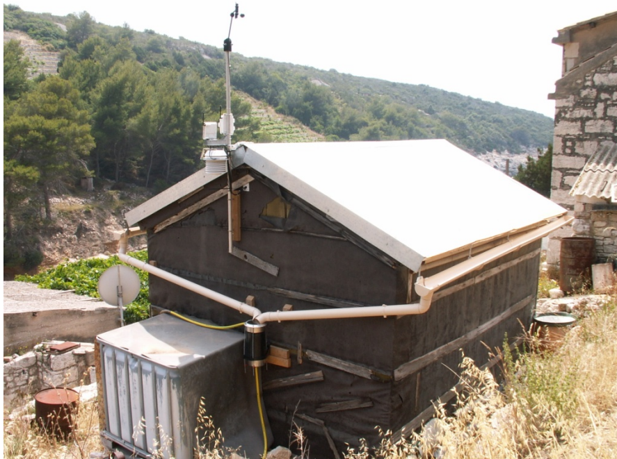
Figure 2: Real life implementation of a dew collection system
