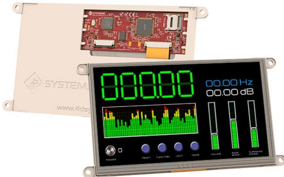
Figure 19: 4D Systems GEN4-ULCD-70DT
