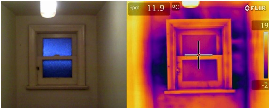
Figure 12: Cold air leaking through behind window trim(Alter, 2014)
