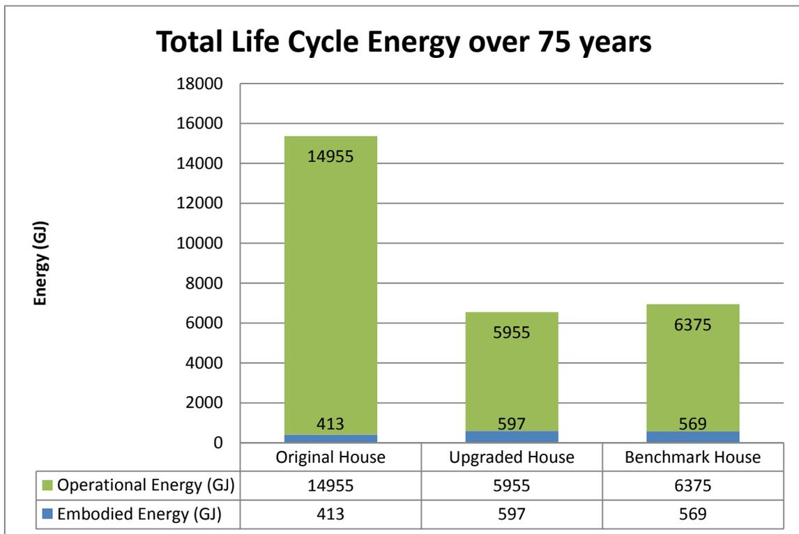
Figure 7 Life Cycle Energy of Original - Historic with no upgrades, Upgraded - Historic with upgrades, and Benchmark - New construction built to code
