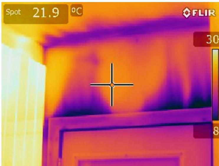
Figure 13: Cold air leaking above well insulated door (Alter, 2014)
