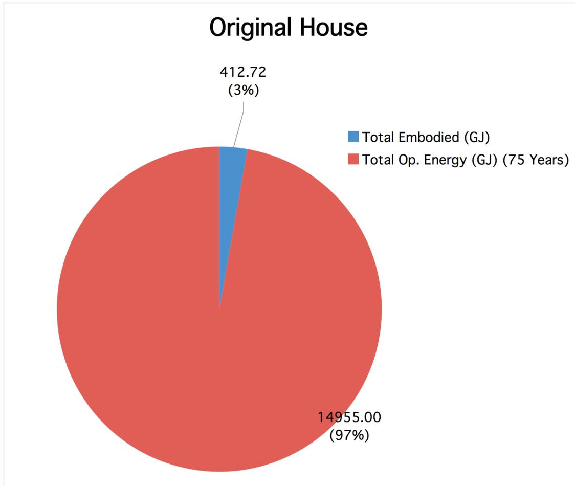
**Figure 2: Original House: Embodied Energy versus Operating Energy (75 years)**
