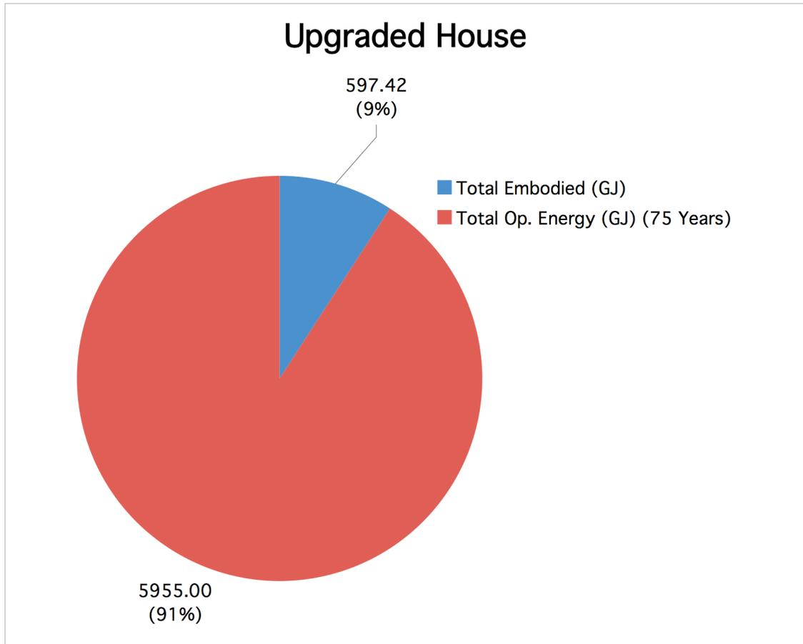
**Figure 3: Upgraded House: Embodied Energy versus Operating Energy (75 years)**
