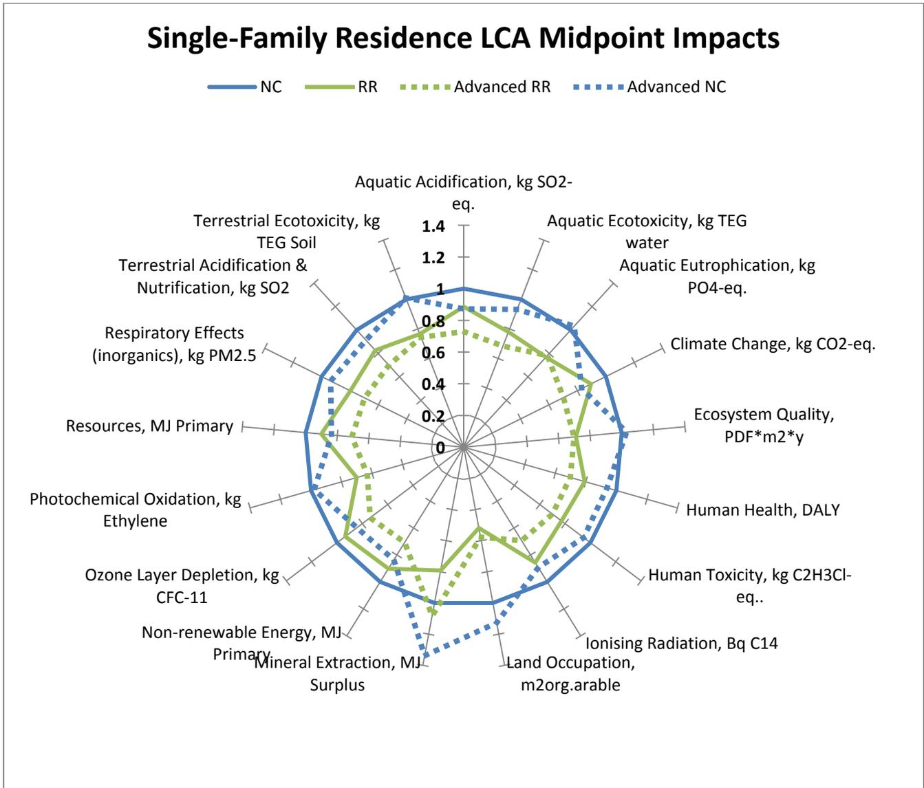
Figure 11: Spider Graph Normalized to Base Case New Construction
