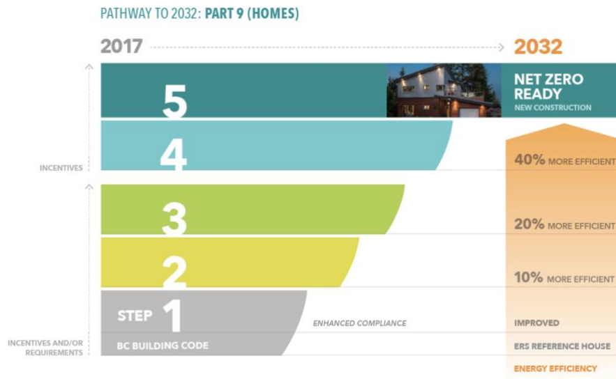
Figure 2: The BC Energy Step Code is divided into 5 steps. The lower steps are easier to achieve while the upper steps are more ambitious.
