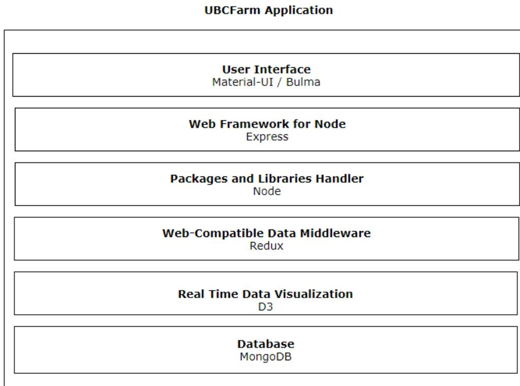
**Figure 1 - Layered Component Diagram**
