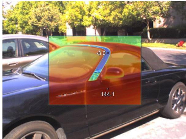
Figure 2. Infrared radiation reflected off a chrome strip. Image: MoistureView.<sup>2</sup>
