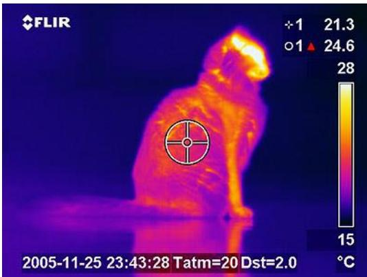
Figure 8. The true temperature of a target can only be estimated using a thermal camera if its emissivity coefficient is known. Image: FLIR.<sup>8</sup>
