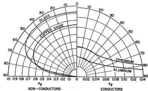
Figure 5. The effect of the angle of incidence on the perceived emissivity of various materials. Note how, when viewed between 80 and 90°, the emissivity of glass is lower than 0.50, while it rises to above 0.90 at a perpendicular angle. Image: MoistureView.<sup>5</sup>
