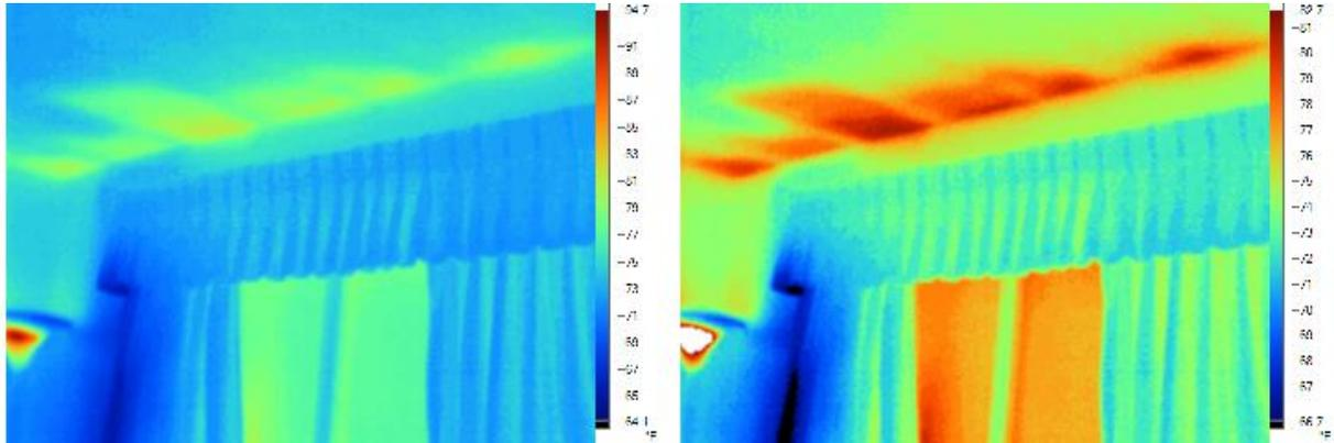
Figure 9. Two thermal images of a room with a light fixture and a large window. Although the scene is identical and the colour gradient is the same, the instrument's readings are displayed using different temperature spans. Image: Thermal Imaging Blog.<sup>9</sup>
