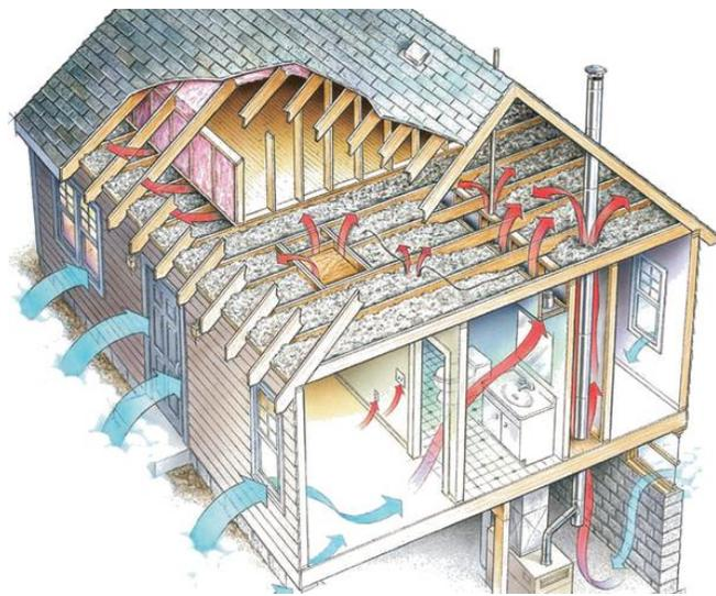
Figure 7. Warm air rises through a building, while cool convective air currents infiltrate through the gaps in the structure’s air barrier. Image: All In One Insulation.<sup>7</sup>
