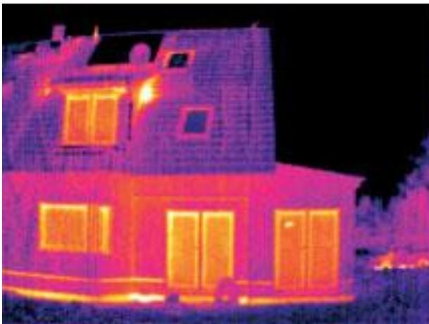
Figure 10. Different materials are used for this house's roof, outer walls, windows and frames. Since each material possesses a distinct emissivity coefficient, the relative temperatures of these materials cannot be compared using a single thermal image. Image: Vollmer & Möllmann, 2010.<sup>10</sup>
