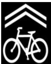
Figure 2. Reference the Auckland study for the specific type of 'sharrow' markings that are painted on the road in the Auckland study.
