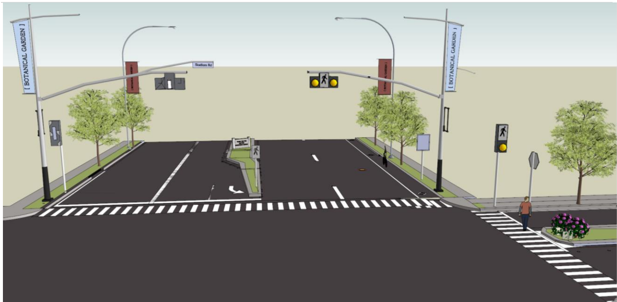
Figure 5 - Conceptual Model of Pedestrian Activated Lights at Stadium St & SW Marine Drive
