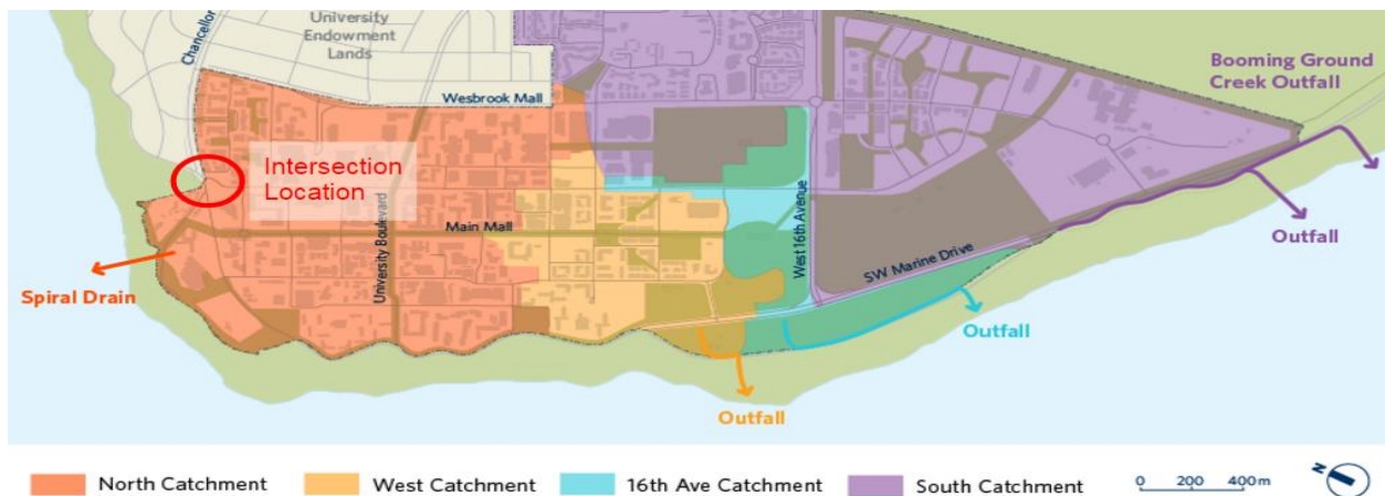
Figure 4. UBC Storm Sewer and Catchment Outfalls Map
