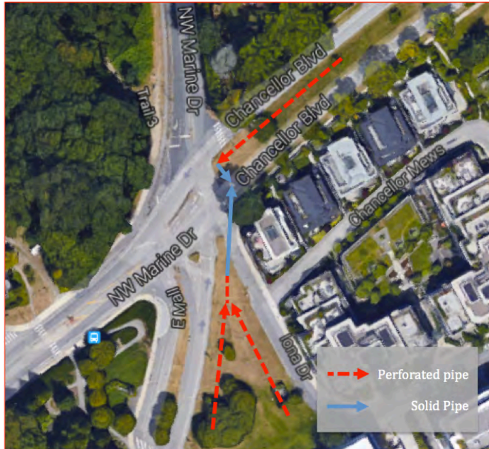
Location of Perforated Pipes
