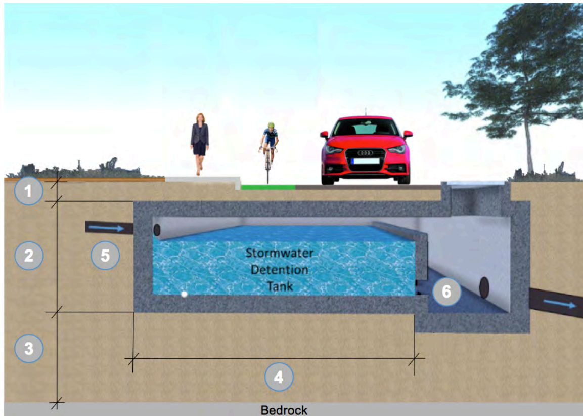
Figure 11 – Cross-sectional View of Stormwater Detention Tank
