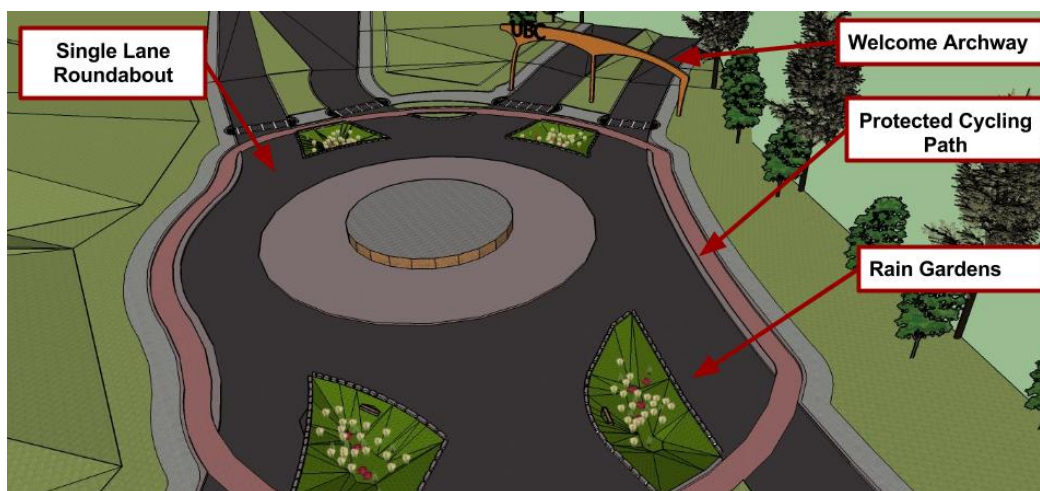
Figure 1: Overview of Key Design Components
