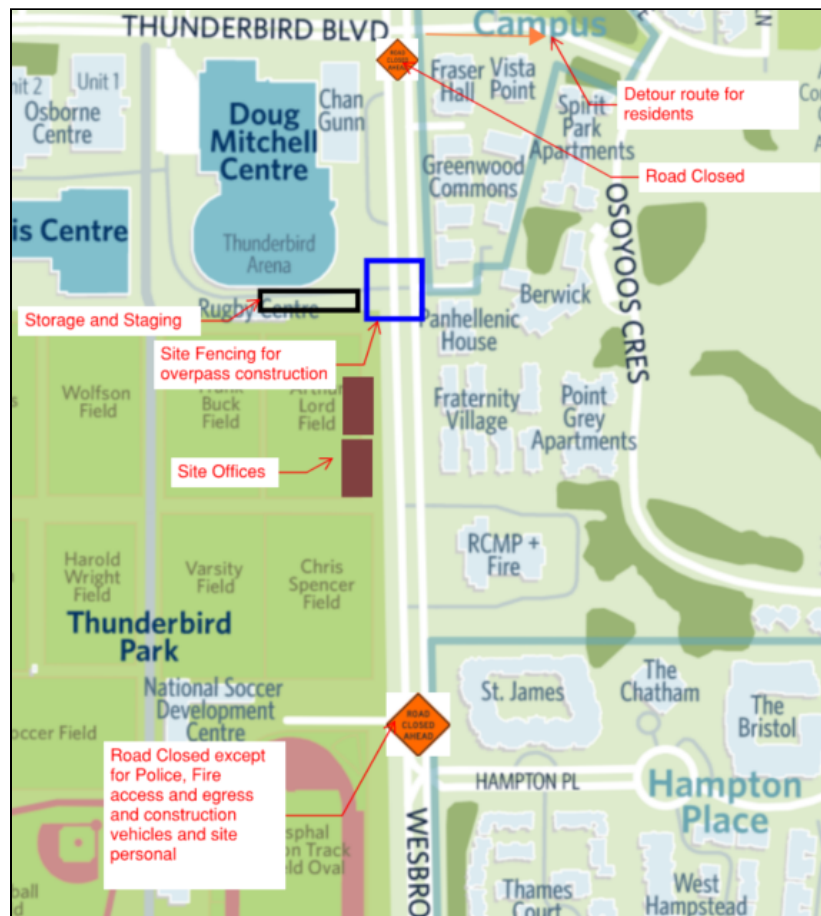
Figure 5.2: Pedestrian Overpass Construction Site Plan and Proposed Detour Route
