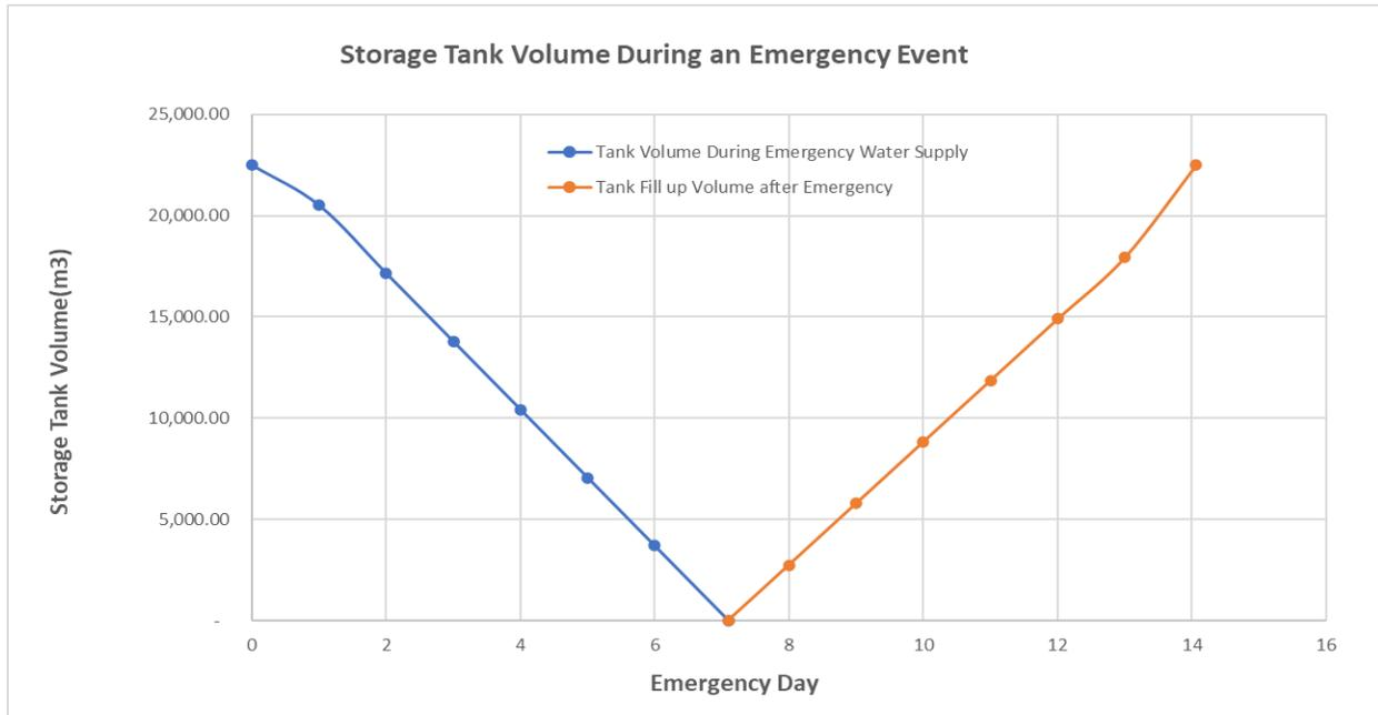
Figure 2. Storage Tank Volume during Emergency Event
