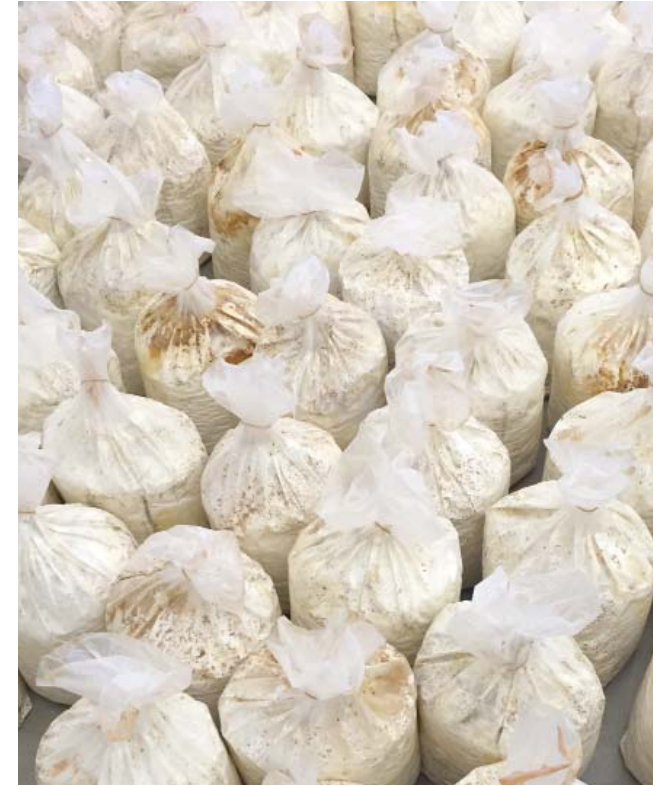
above and below: Block production. After sterilization, inoculation, and incubation, colonized substrates are moulded in batches to produce durable living blocks.
