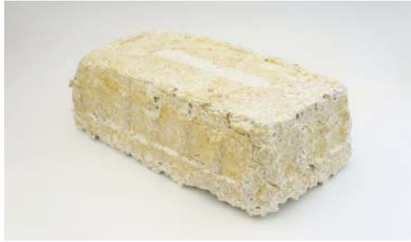
above and below: Block production. After sterilization, inoculation, and incubation, colonized substrates are moulded in batches to produce durable living blocks.
