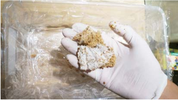
above and below: Block production. After sterilization, inoculation, and incubation, colonized substrates are moulded in batches to produce durable living blocks.
