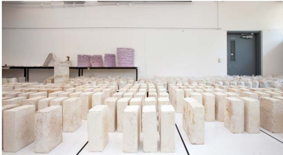
above and below: Block production. After sterilization, inoculation, and incubation, colonized substrates are moulded in batches to produce durable living blocks.
