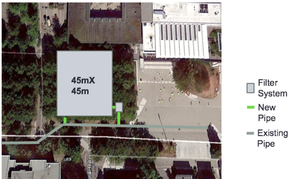
Figure 7b) First Detention Tank - By the SUB Building – Plan View
