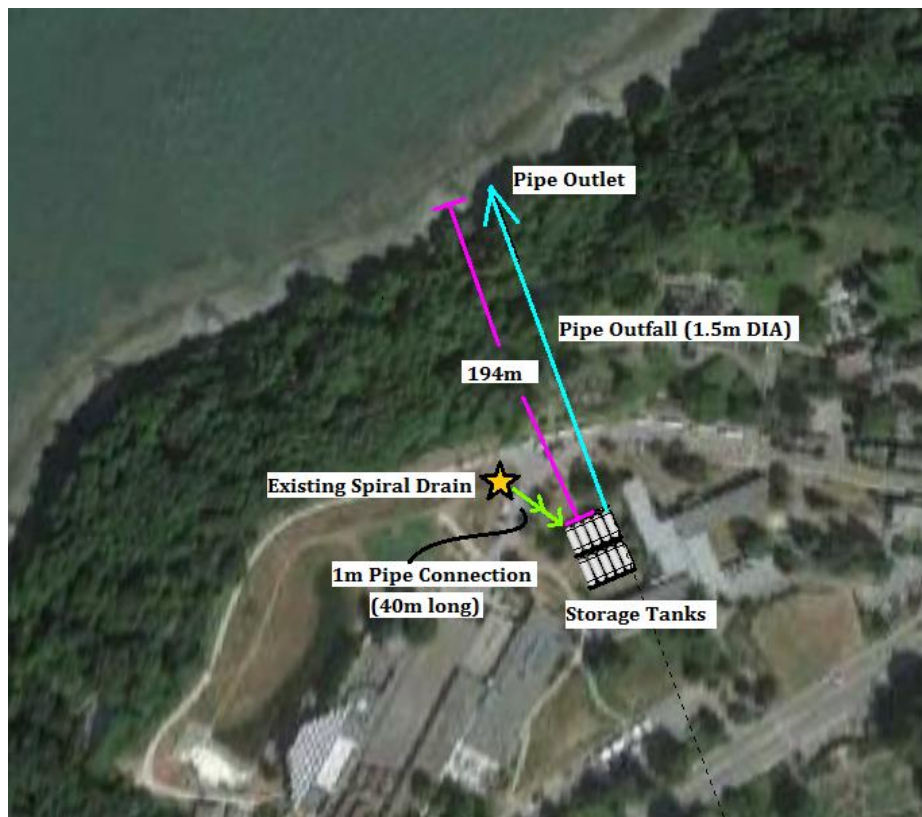
Figure 14: Orientation of Storage Tanks
