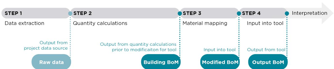
Figure 4: BoM generation process and the BoMs produced in each step
