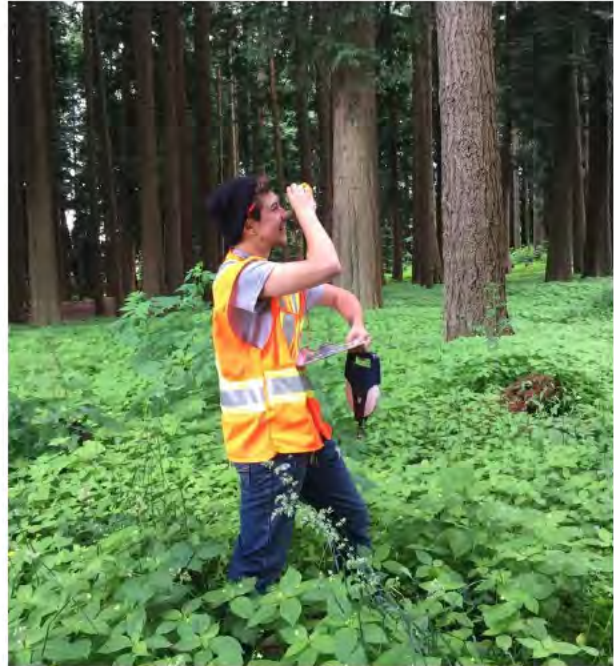
Image 3. Using a clinometer to record the top angle
