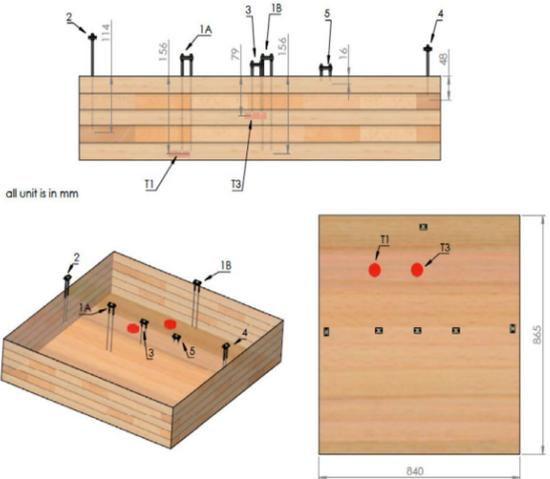
Figure 1: Location of the moisture content and temperature sensors within a CLT panel.
