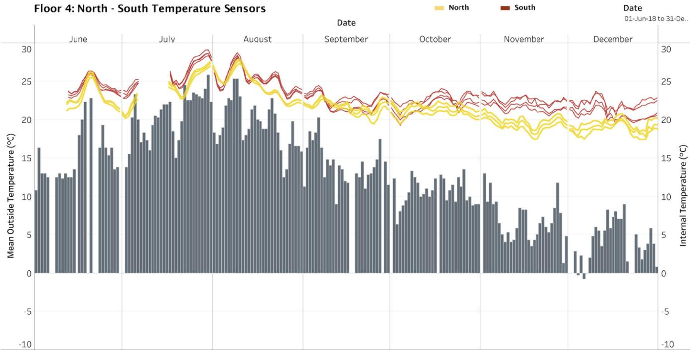
Figure 22 : Floor 4: North - South Temperature Sensors. The internal temperature of the CLT panels against the average outside temperature, comparing the measured values in Floor 4 in North-South locations. (X-axis - Days from June 1, 2018, to December 31, 2018; Dual Y-axis- Left: Outside temperature in °C and Right: Internal temperature in °C)
