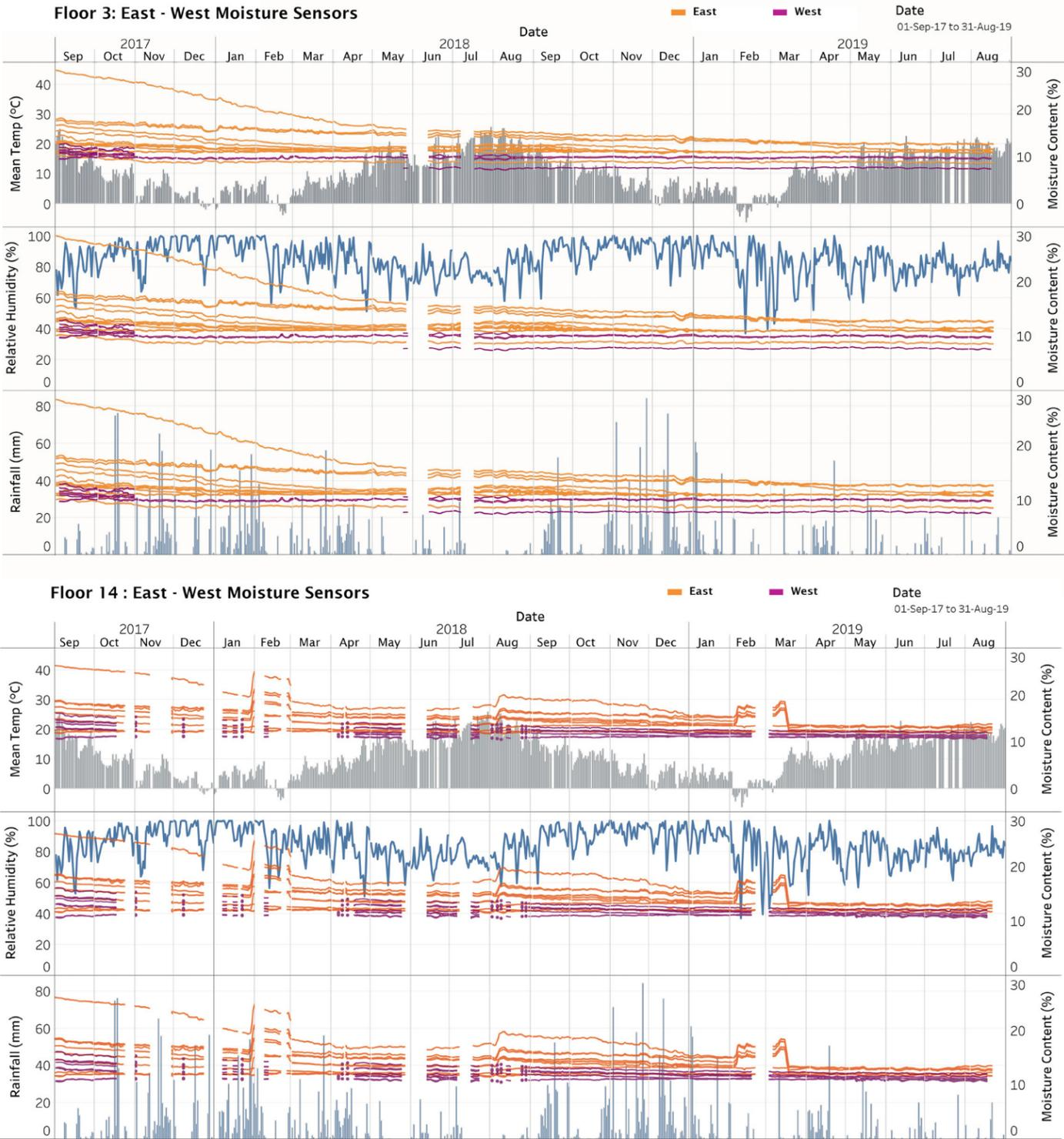
Figure 12: Floor 3: East - West Moisture Sensors. The moisture content of the CLT panels and its relation to the orientation, by comparing the data from the East and the West sensors at Floor 3. (X-axis - Days from September 1, 2017, to August 31, 2019; Dual Y-axis- Left: Climate conditions and Right: Moisture content values in %)
