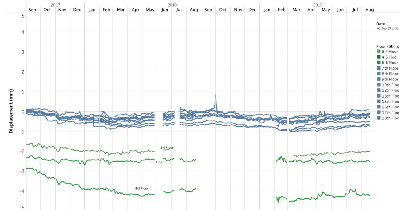
Figure 24 : Vertical movement recorded by the string pot sensors installed on each floor for the days between September 1, 2017, and August 31, 2019.
