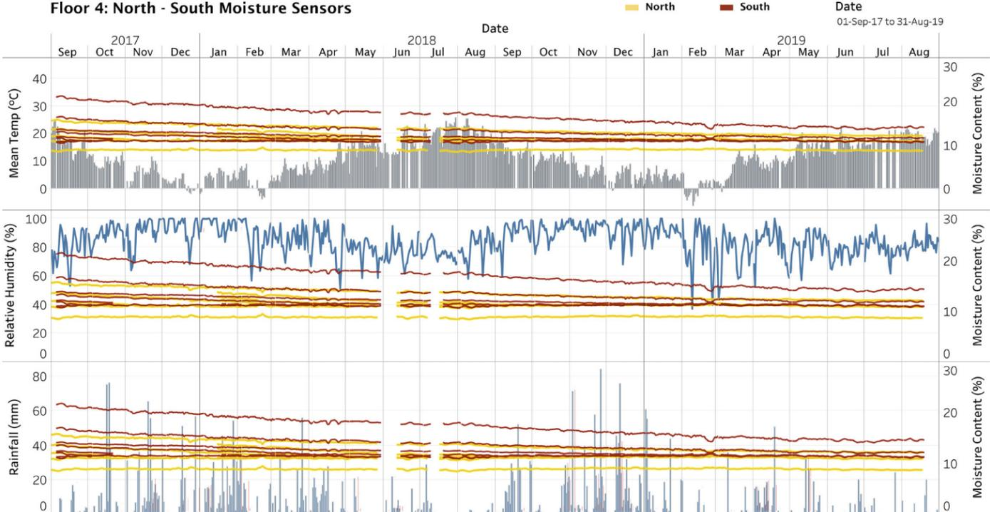
Figure 14: Floor 4: North-South Moisture Sensors. The moisture content of the CLT panels and its relation to the orientation, by comparing the data from the North and the South sensors at Floor 4. (X-axis - Days from September 1, 2017, to August 31, 2019; Dual Y-axis- Left: Climate conditions and Right: Moisture content values in %)
