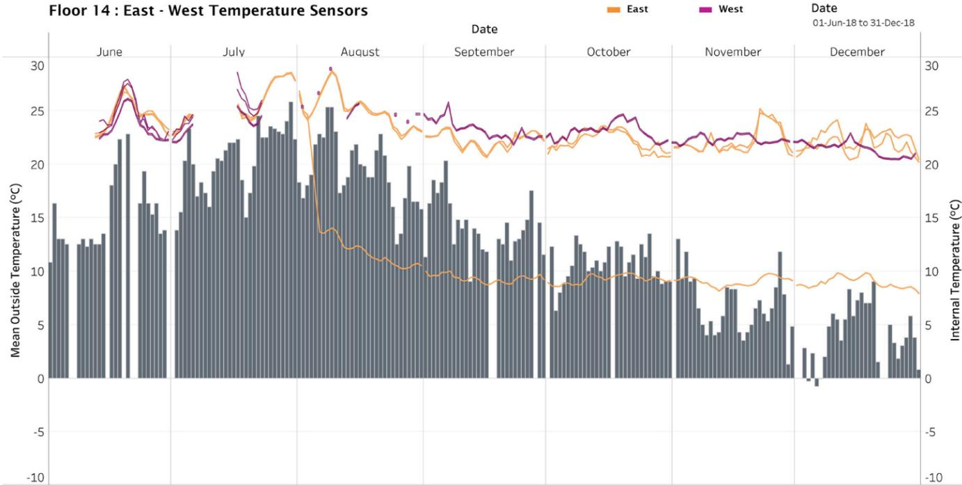
Figure 21 : Floor 14: East - West Temperature Sensors. The internal temperature of the CLT panels against the average outside temperature, comparing the measured values in Floor 14 in East-West locations
