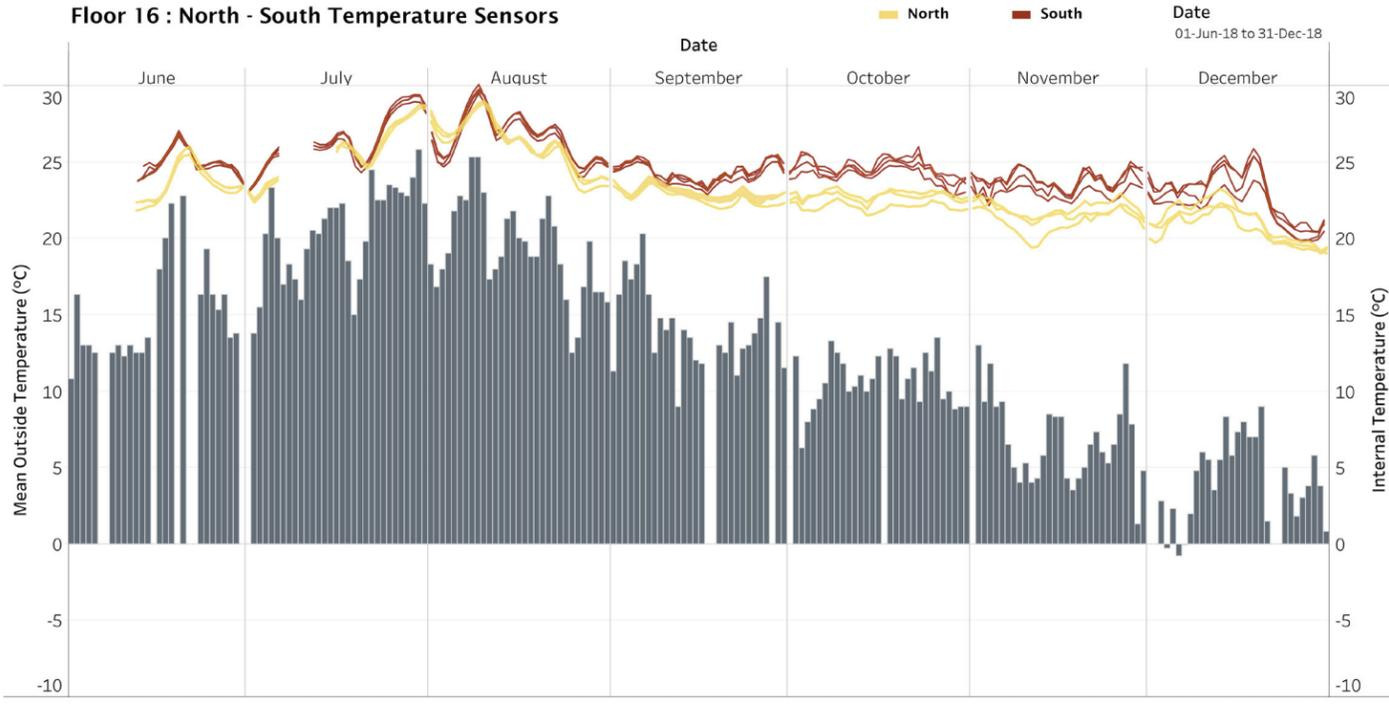
Figure 23 : Floor 16: North - South Temperature Sensors. The internal temperature of the CLT panels against the average outside temperature, comparing the measured values in Floor 16 in North-South locations. (X-axis - Days from June 1, 2018, to December 31, 2018; Dual Y-axis- Left: Outside temperature in °C and Right: Internal temperature in °C)
