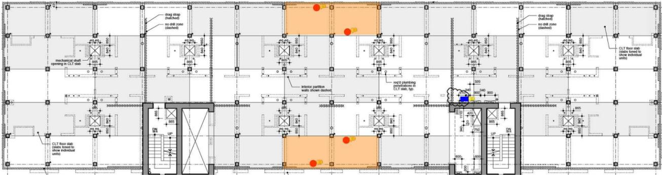
Figure 3 : Location of the moisture content and temperature sensors installed CLT panels on each floor. (LEFT: East-West moisture monitoring sensors, RIGHT: North-South moisture monitoring sensors)
