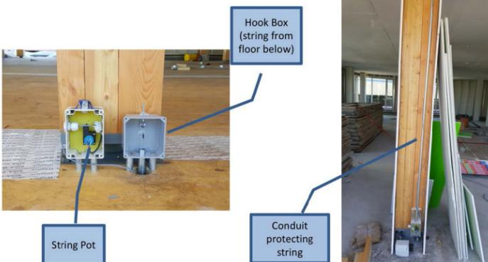
Figure 2: Arrangement of the string pot sensors along the columns.
