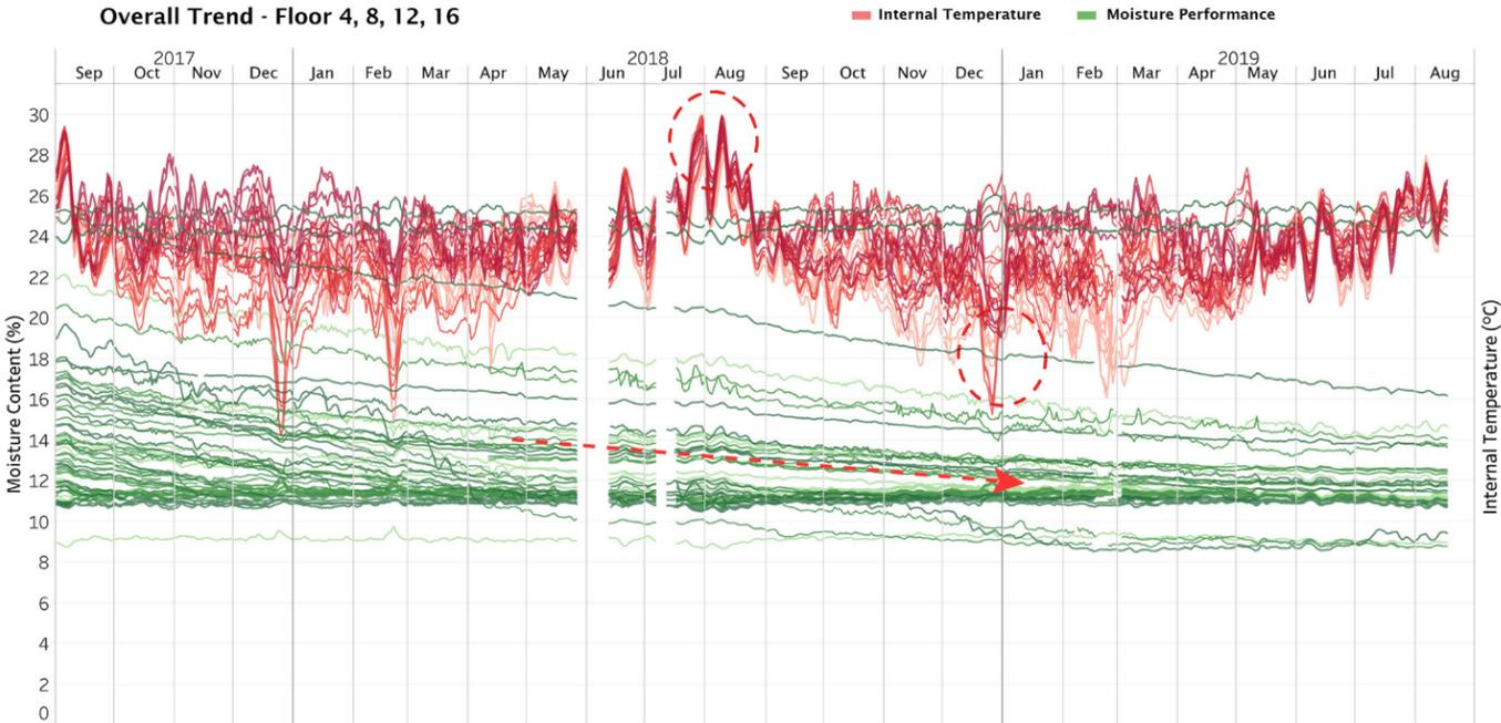
Figure 5: Overall Trend - Floor 4, 8, 12, 16. The moisture content and internal temperature of the CLT panels plotted against the period from September 1, 2017, to August 31, 2019 for sensors at Floor 4, 8, 12, 16 that were sourced from North-South locations.
