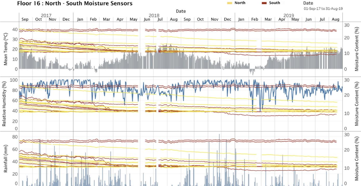
Figure 15: Floor 16: North-South Moisture Sensors. The moisture content of the CLT panels and its relation to the orientation, by comparing the data from the North and the South sensors at Floor 16. (X-axis - Days from September 1, 2017, to August 31, 2019; Dual Y-axis- Left: Climate conditions and Right: Moisture content values in %)
