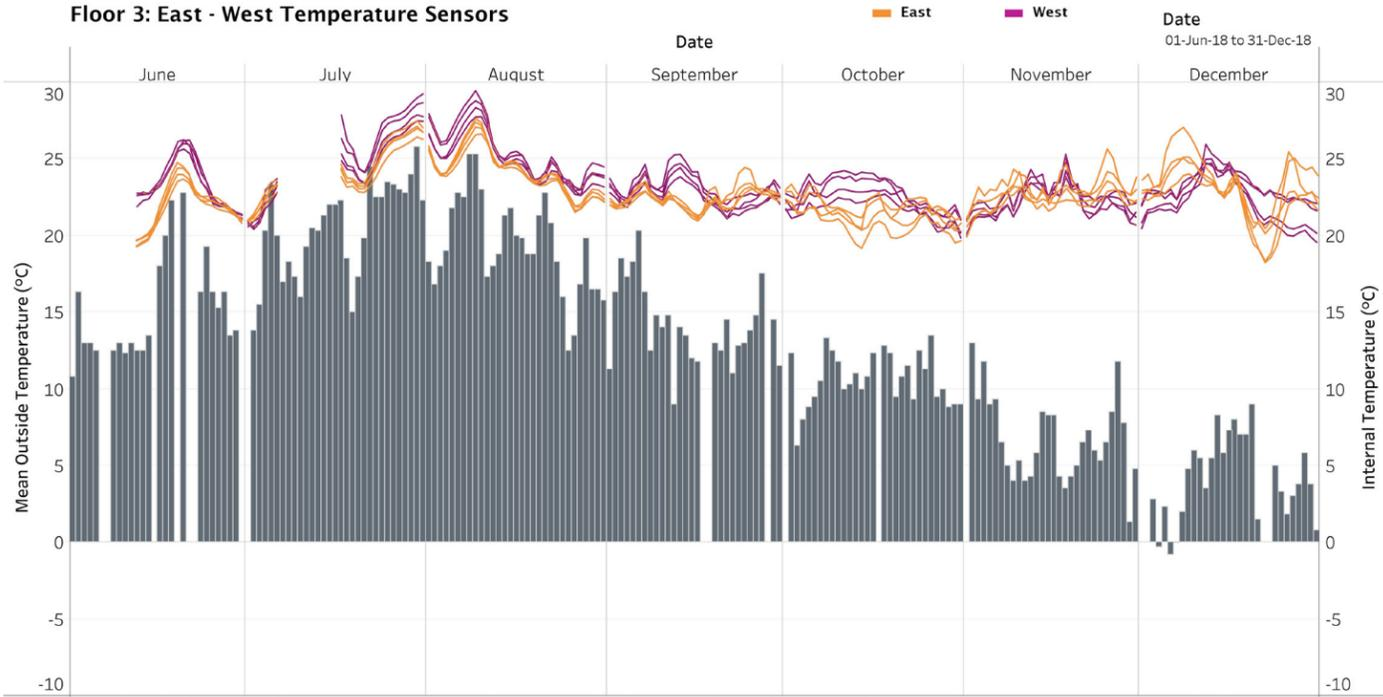
Figure 20 : Floor 3: East - West Temperature Sensors. The internal temperature of the CLT panels against the average outside temperature, comparing the measured values in Floor 3 in East-West locations.
