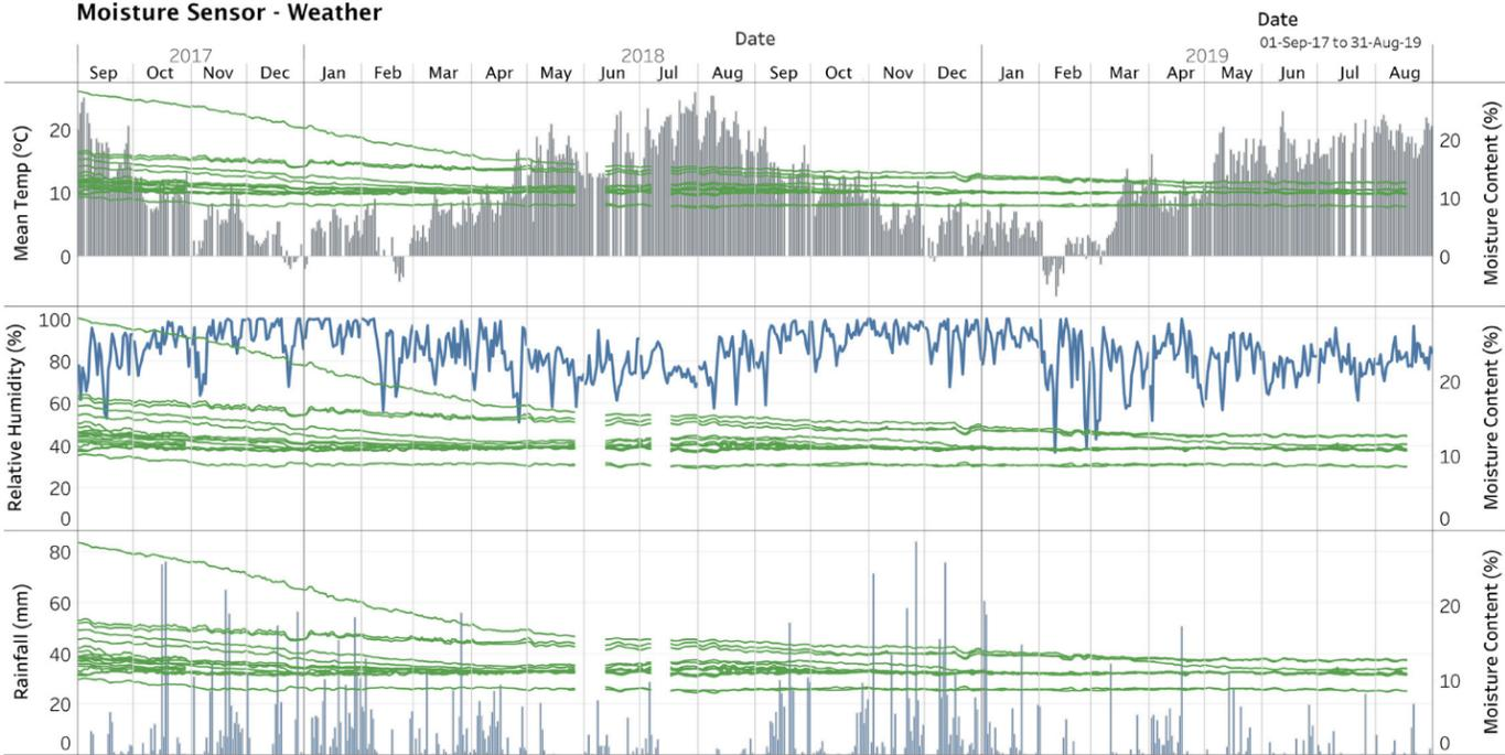
Figure 6: Moisture Sensor - Weather. The moisture content of the CLT panels in Floor 3 and its relation to external climate conditions (X-axis - Days from September 1, 2017, to August 31, 2019; Dual Y-axis- Left: Climate conditions and Right: Moisture content values in %)
