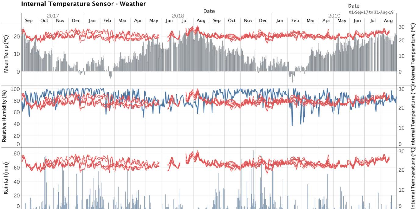
Figure 7: Internal Temperature Sensor - Weather. The internal temperature of the CLT panels in Floor 3 and its relation to external climate conditions. (X-axis - Days from September 1, 2017, to August 31, 2019; Dual Y-axis- Left: Climate conditions and Right: Internal Temperature values in °C)
