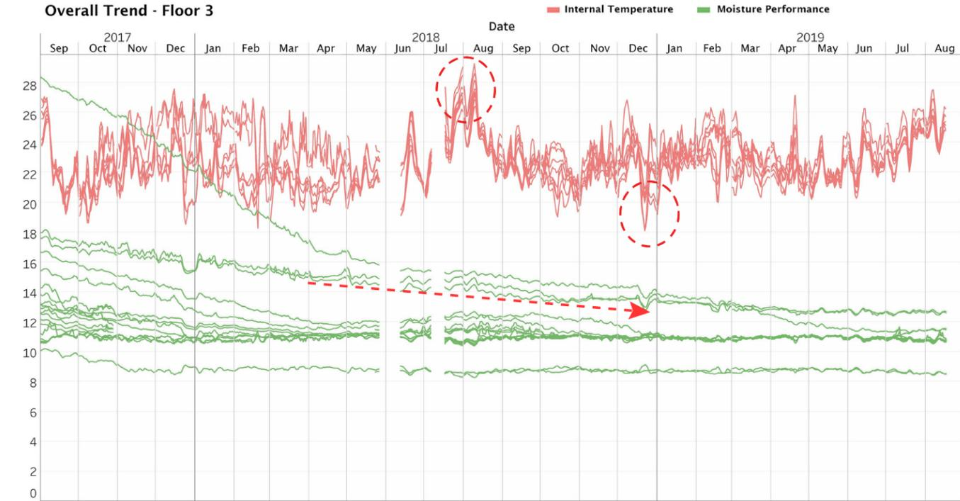
Figure 4: Overall Trend - Floor 3. The moisture content and internal temperature of the CLT panels plotted against the period from September 1, 2017, to August 31, 2019 for sensors at Floor 3, sourced from East-West locations.
