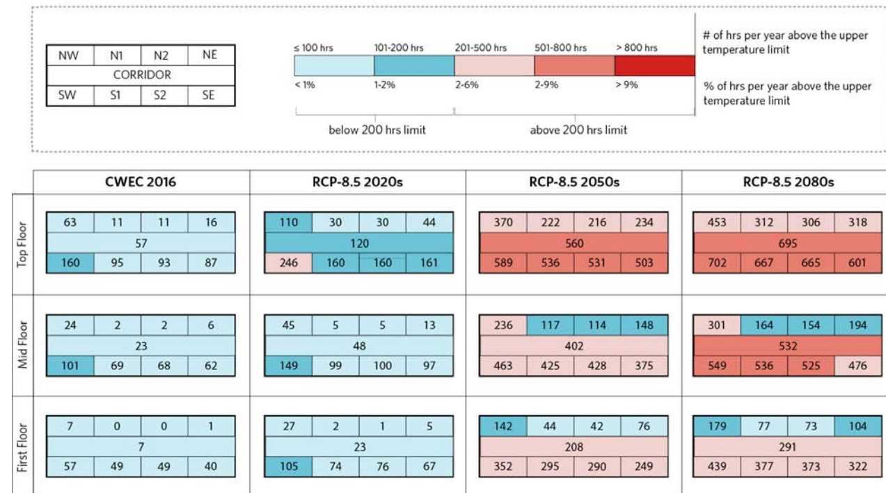
Figure 2. The number of overheated hours for a new low-rise building, with CAMMs designed to Step 3 requirements, in the CWEC 2016, RCP-8.5 2020s, 2050s and 2080s climate scenarios.
