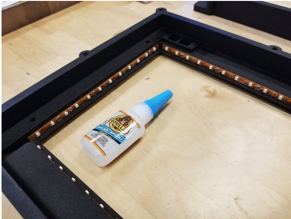
Figure 8. Enclosure with LED Strip Adhered
