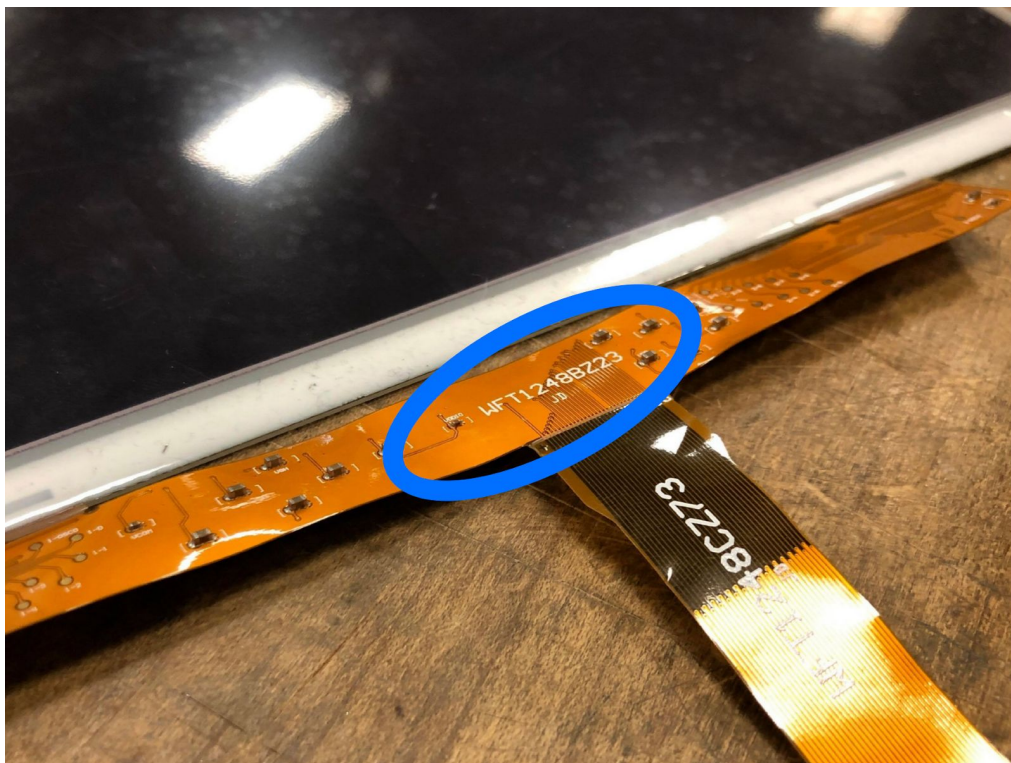
Figure 30. Serial Location on FPC
