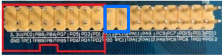
Figure 31. Connector Locations (Blue - Pins Removed)
