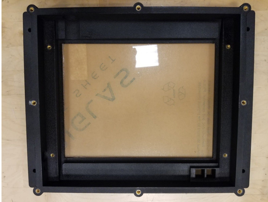
Figure 14. Enclosure with Heat-Set Inserts
