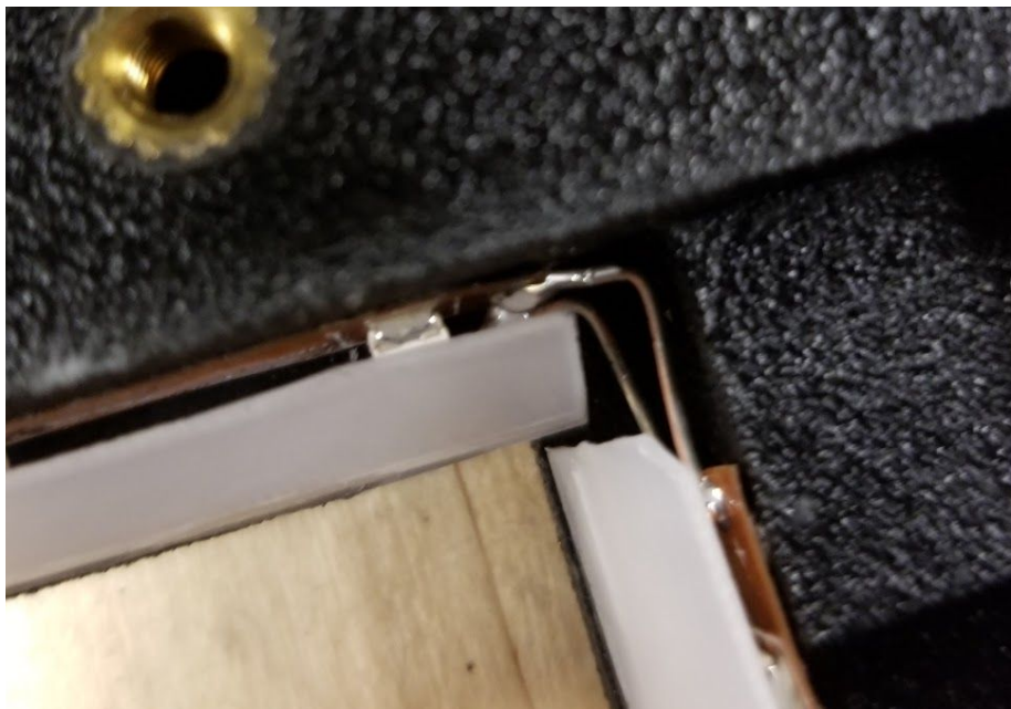
Figure 10. Connections Between LED Strips
