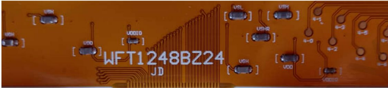
Figure 29. Ancillary FPC with Connector P2
