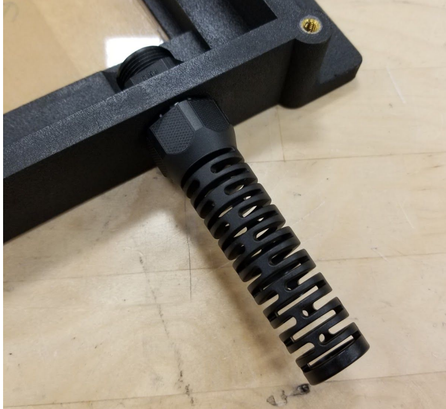
Figure 16. Installed Cable Gland
