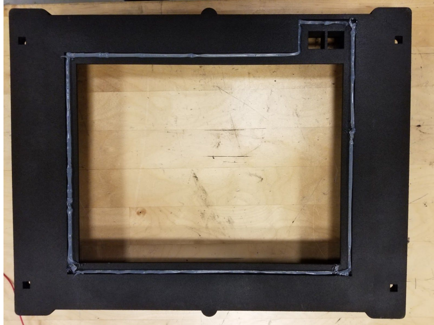
Figure 12. Enclosure with Silicone Adhesive Applied
