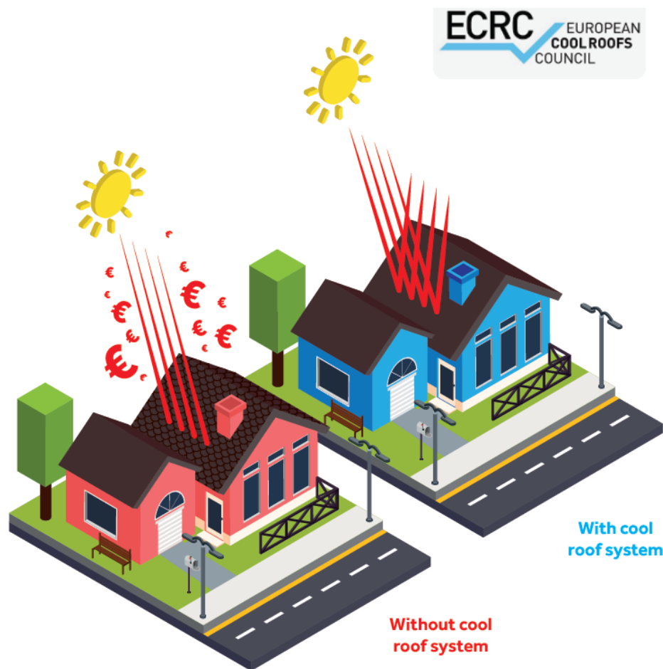
Figure 5 A typical cool roof system. A Cool Roofing product shows higher solar reflectance compared to other conventional roof materials of the same color (BIM International, 2025).
