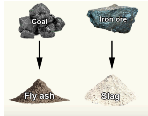
Figure 12. Green Concrete with SCMs substitution (Image source: https://turritopsis.org/en/author/rachid/ ; https://www.facebook.com/EMSPetrography/posts/add-ons-to-your-cement-supplementary-cementitious-materials-or-scms-are-fine-gra/166490525077950/ )
