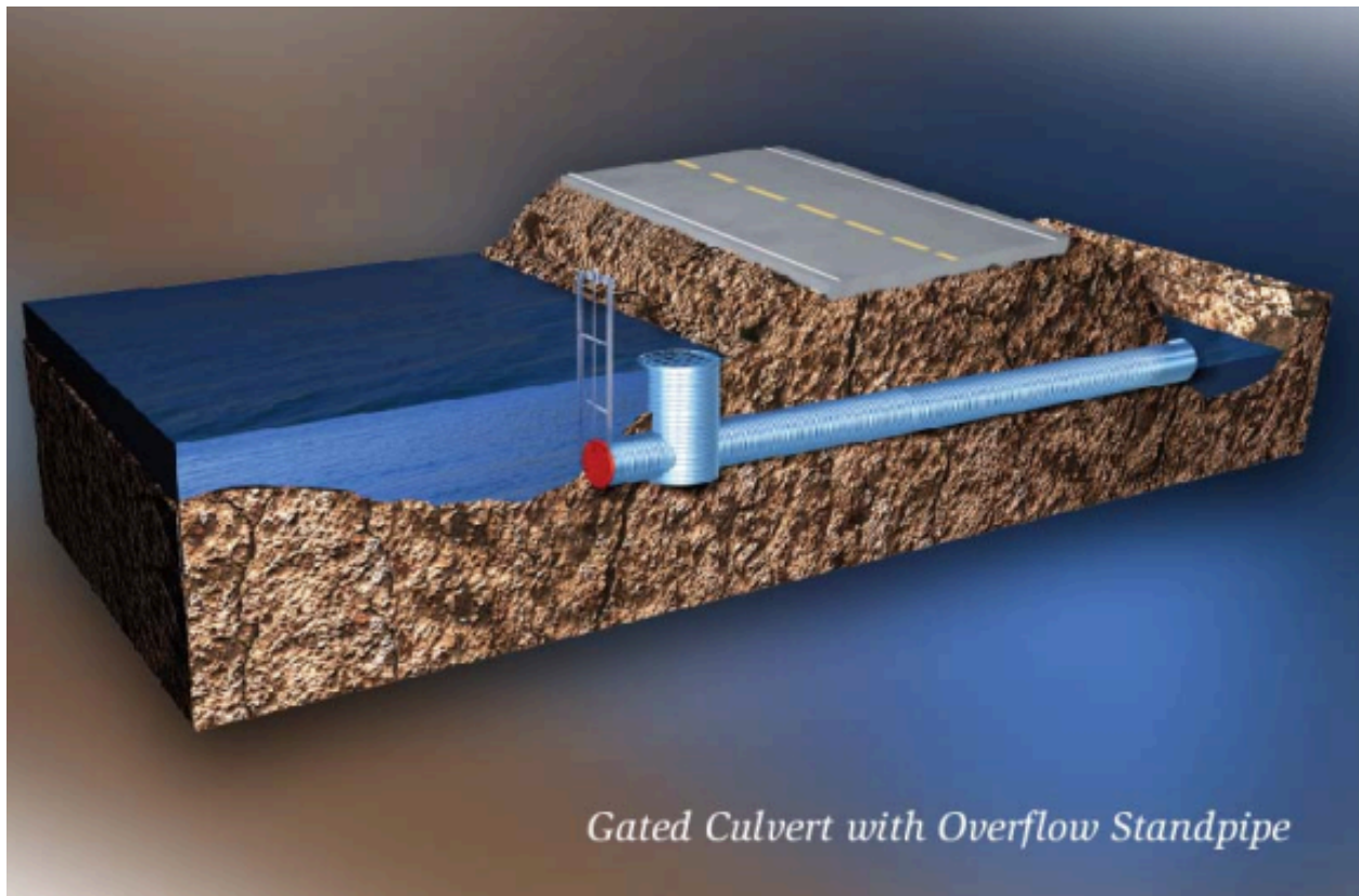
Figure 3: A gated culvert uses gravity to distribute flood waters from the waterway to a retention area. The raised road contains the water to be temporarily stored until it can be slowly released slowly back into the river.
