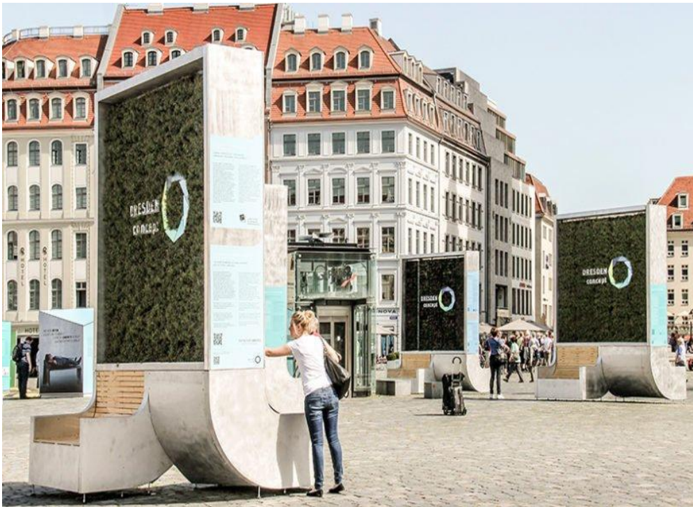
Figure 69: The City Tree, an urban air purifier that incorporates seating
