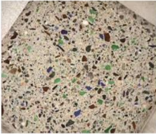
Fig. 5.7 Use of glass aggregate in concrete
