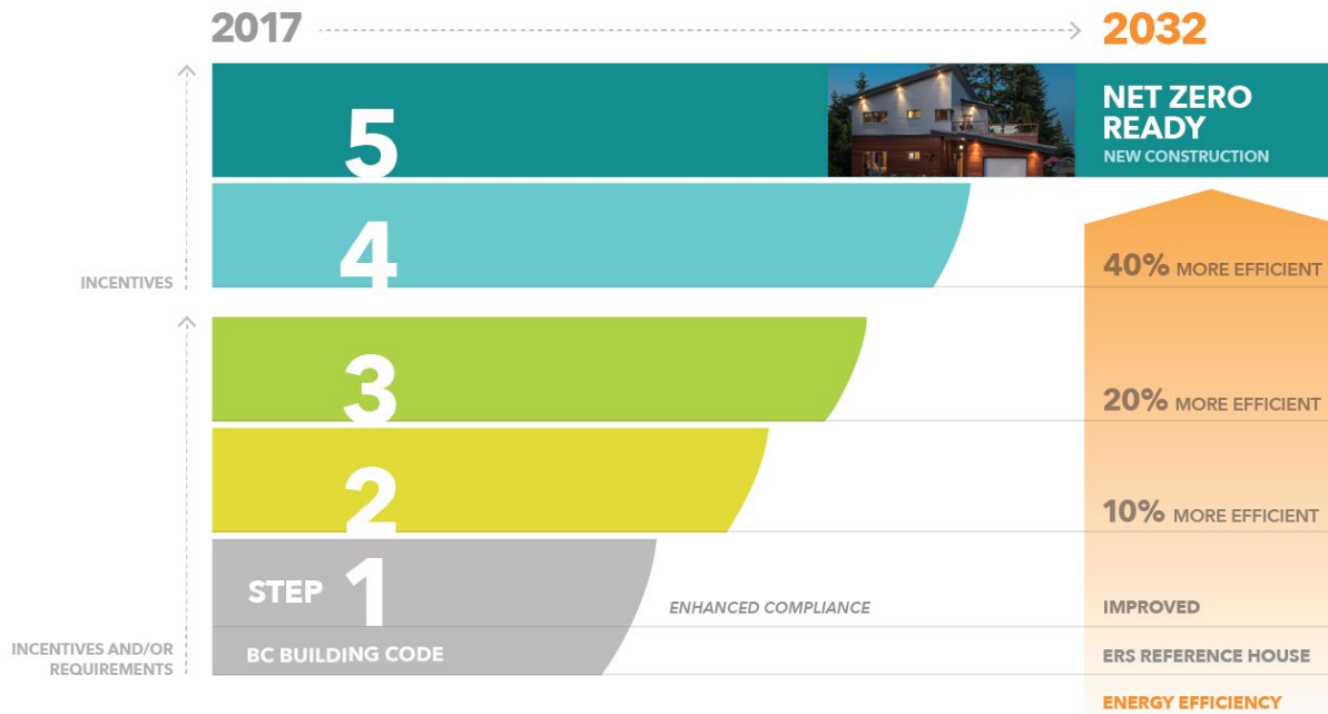
Figure 4: BC Energy Step Codes Steps for Part 9 Homes (From Government of BC Building Safety Standards Branch)
