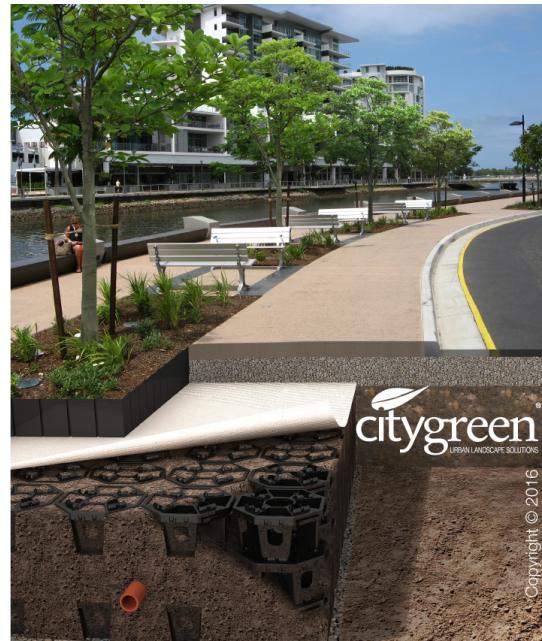
Figure 14 Soil cells for planting in soil strip by curb (illustration by City Green, 2016)
