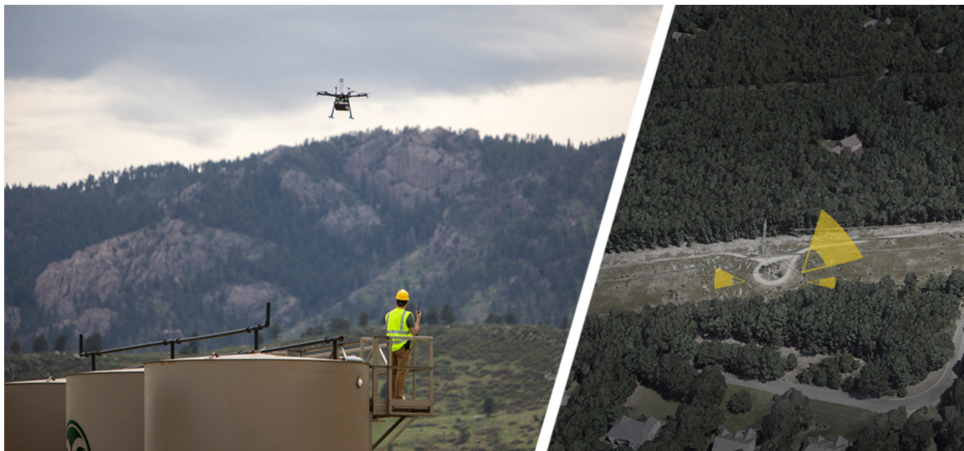
Figure 2. An unmanned gas leak detection system from ULC Robotics (2019). These drones-based leak detection systems can not only measure concentration of methane gas (ppb) in air samples using laser spectroscopy but can also offer information on the leaking sources and rate of leaks 27 .
