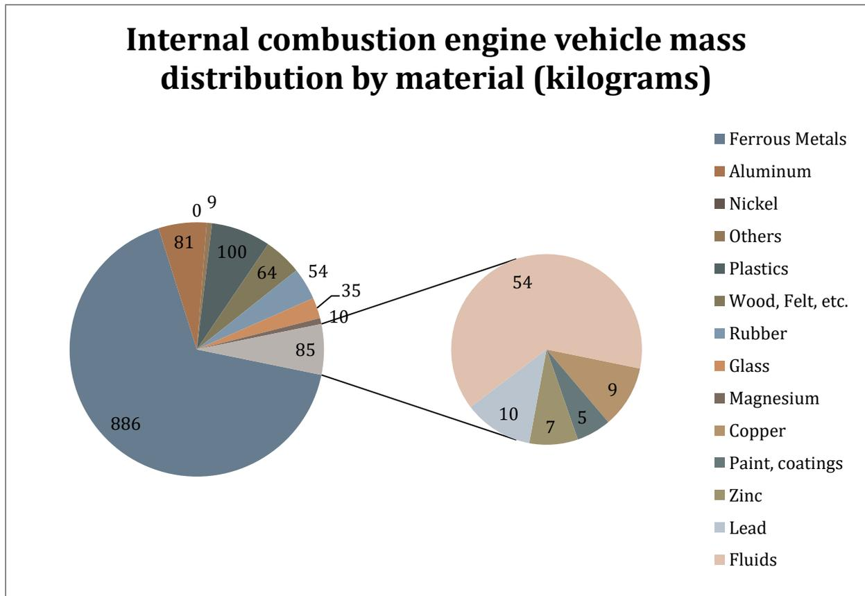
Figure 2 – Mass distribution of an internal combustion engine vehicle. Various alloys of steel account for two thirds (67%) of vehicle mass, with aluminum and plastics having the largest mass for non-steel materials (Weiss & Heywood, 2000).
