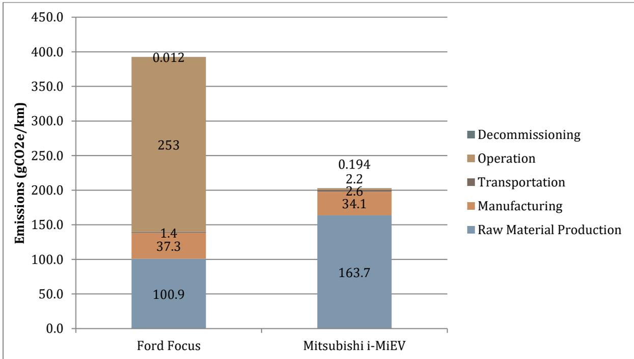
Figure 5 – Graph comparing CO<sub>2</sub>-equivalent emissions with a vehicle life of 150,000km.
