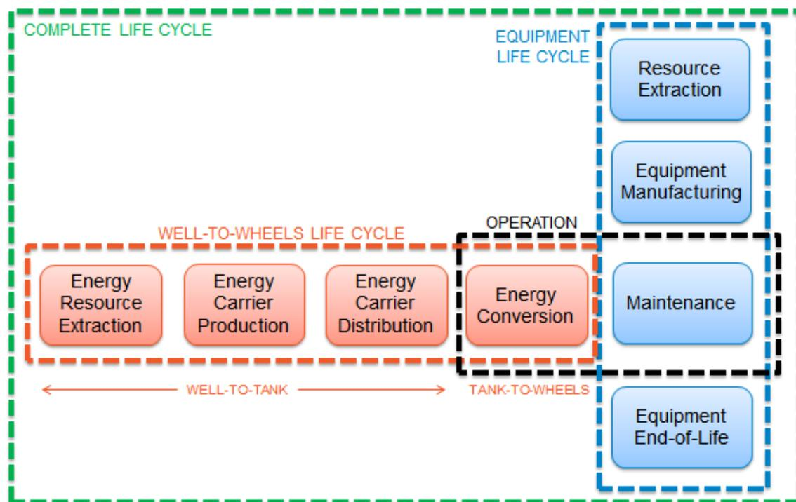
Figure 1 – System boundaries for a complete life cycle analysis of vehicles. This study focuses on the equipment life cycle and does not analyze the well-to-wheels life cycle. (Nordelöf & Messagie, 2014)
