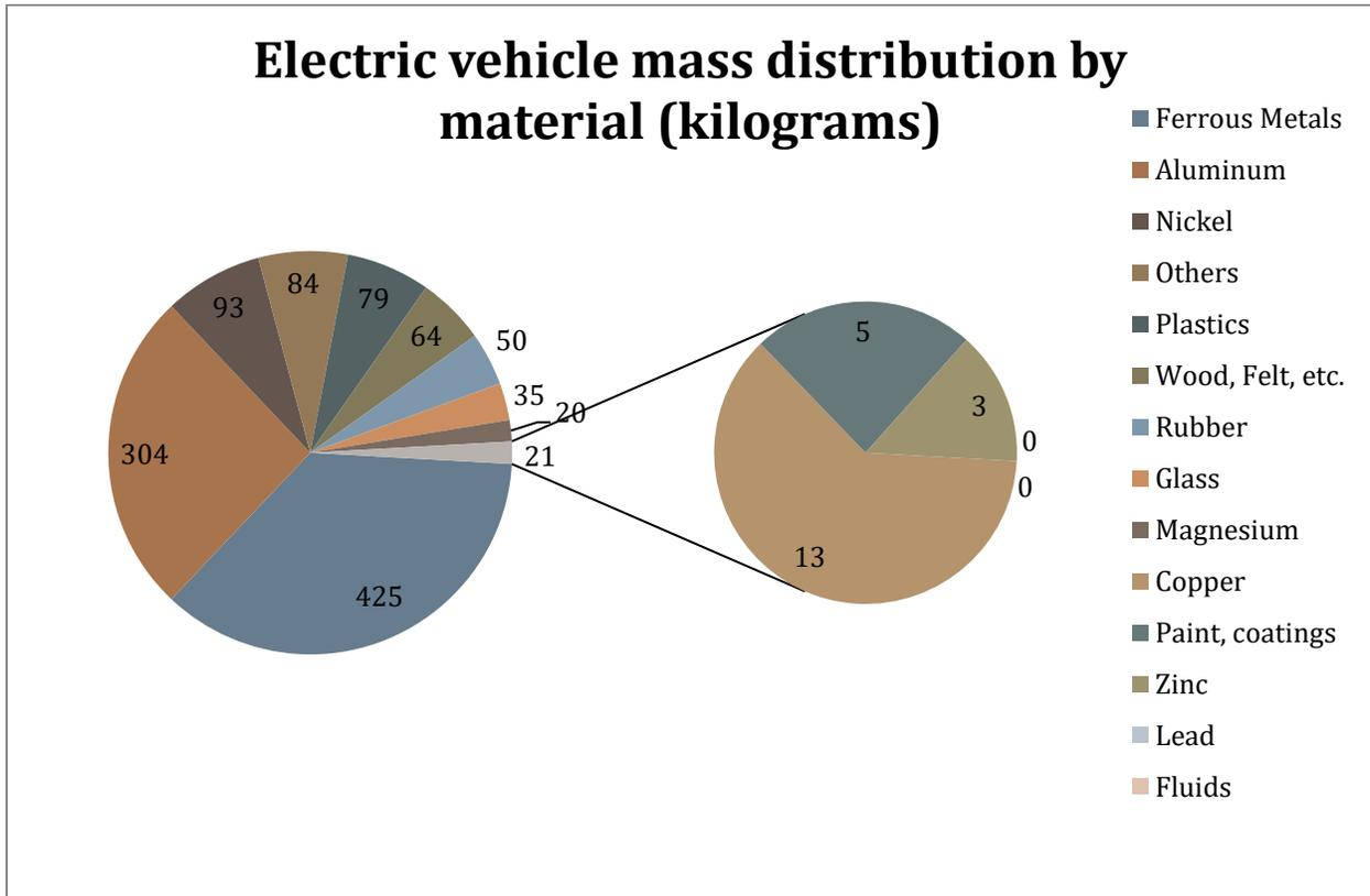
Figure 3 – The predicted mass distribution of an electric vehicle in 2020 shows a different picture, with aluminum and nickel having a much more significant role. Ferrous metals (mainly high-strength steel) are still the dominant material. (Weiss & Heywood, 2000)
