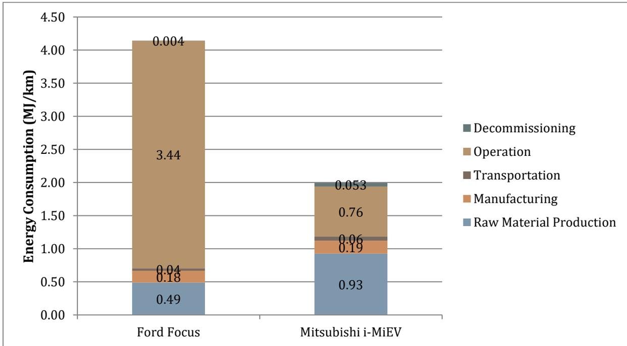
Figure 6 – Graph comparing energy consumption with a vehicle life of 150,000km.
