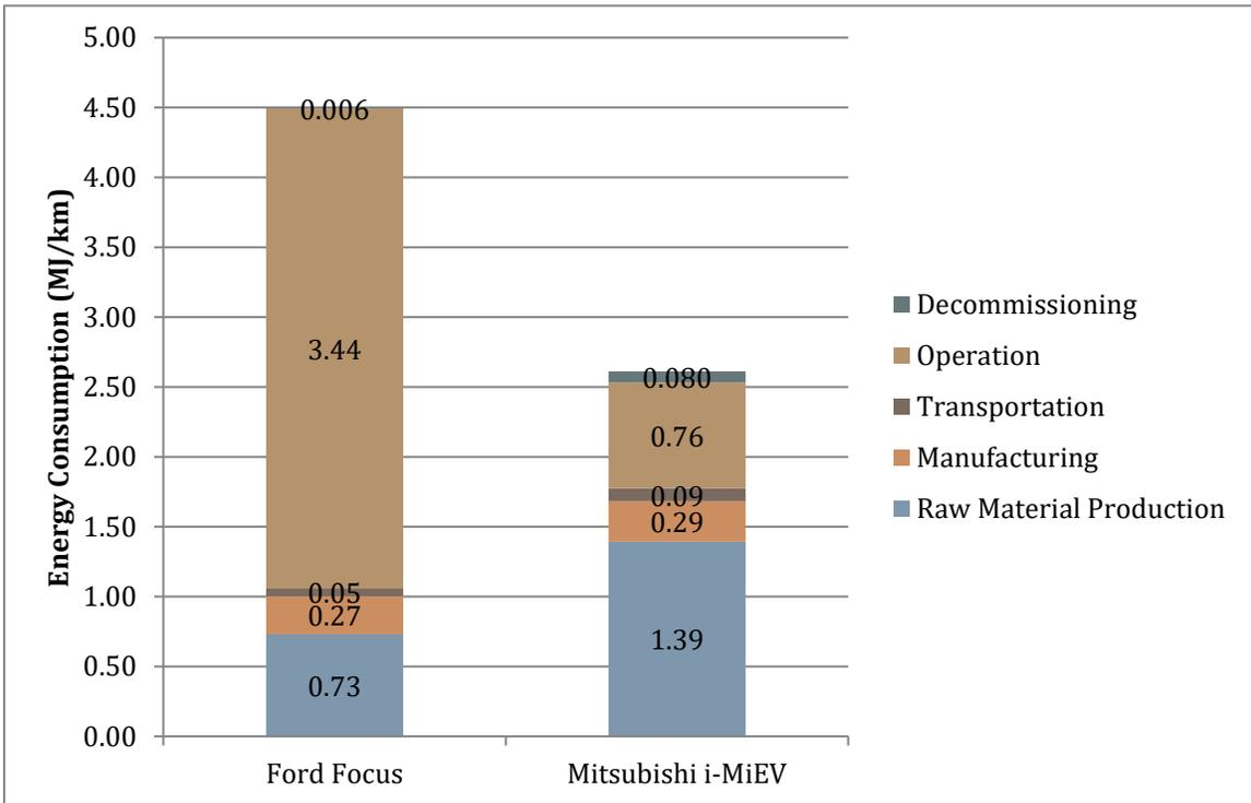
Figure 10 – Graph comparing energy consumption with a vehicle life of 100,000km.
