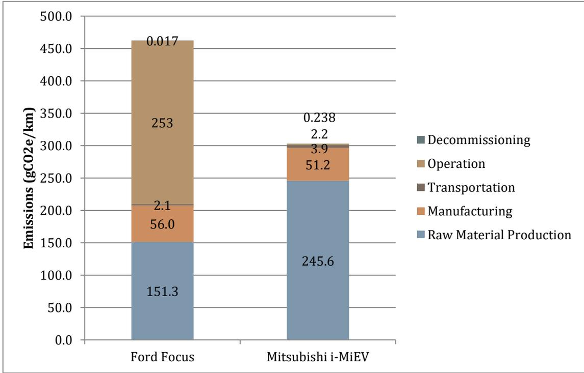
Figure 9 – Graph comparing CO<sub>2</sub>-equivalent emissions with a vehicle life of 100,000km.
