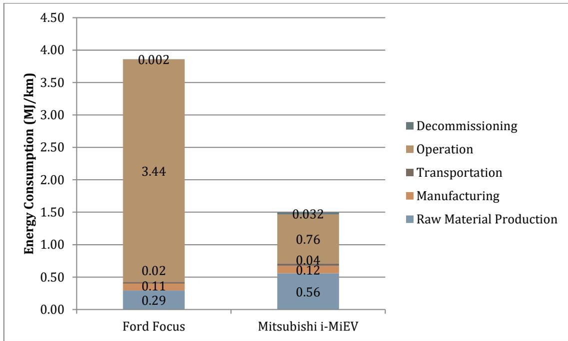
Figure 8 – Graph comparing energy consumption with a vehicle life of 250,000km.
