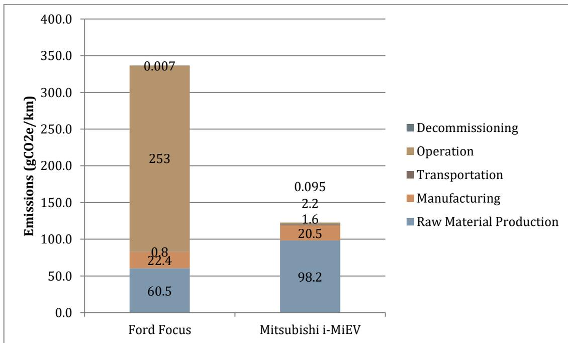
Figure 7 – Graph comparing CO<sub>2</sub>-equivalent emissions with a vehicle life of 250,000km.
