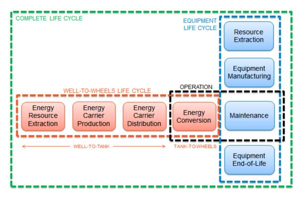
Figure 1 – System boundaries for a complete life cycle analysis of vehicles. This study focuses on the equipment life cycle and does not analyze the well-to-wheels life cycle. (Nordelöf & Messagie, 2014)
