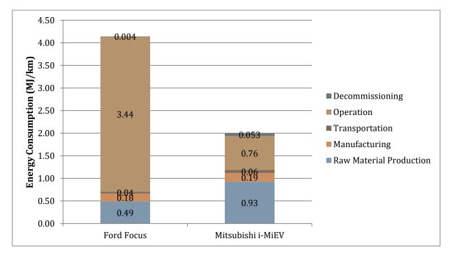
Figure 6 – Graph comparing energy consumption with a vehicle life of 150,000km.
