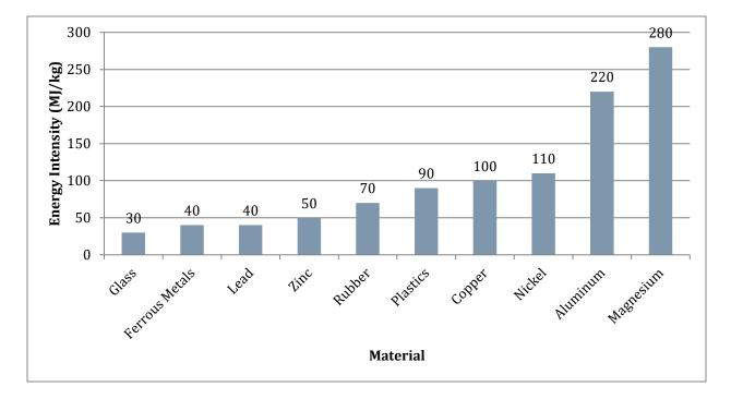
Figure 4 – Graph showing energy required per unit mass to convert various raw materials to usable virgin feedstock for a manufacturing process (Sullivan & Burnham, 2010).
