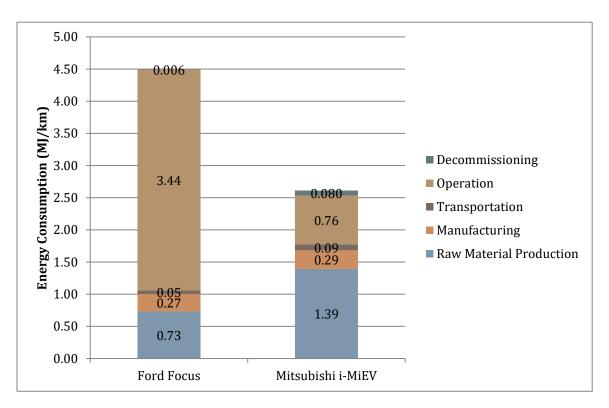
Figure 10 – Graph comparing energy consumption with a vehicle life of 100,000km.
