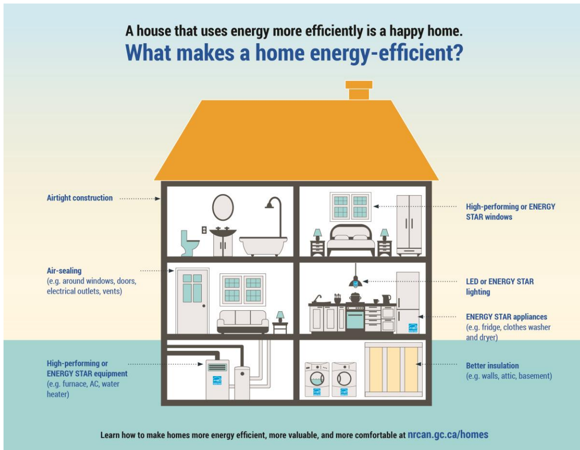
Figure 2: Some Features of an Energy Efficient Home
