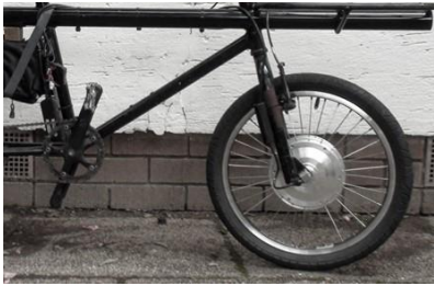
Figure 29: Front hub motor.
