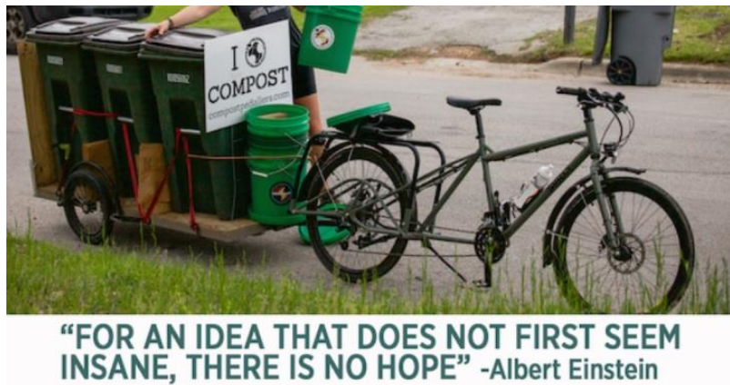
Figure 46: A longtail cargo bicycle with a trailer is being used for compost collection in Austin, USA.
