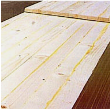
Figure 4. Panel Made from Glued-up Lamells
