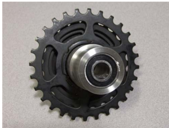
Figure 23: Custom Hub with Cassette and bearings
