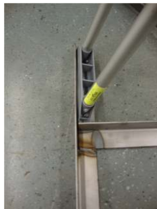
Figure 21: Front Fork Temporarily Located Horizontally
