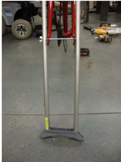
Figure 20: Front Fork Secured Temporarily
