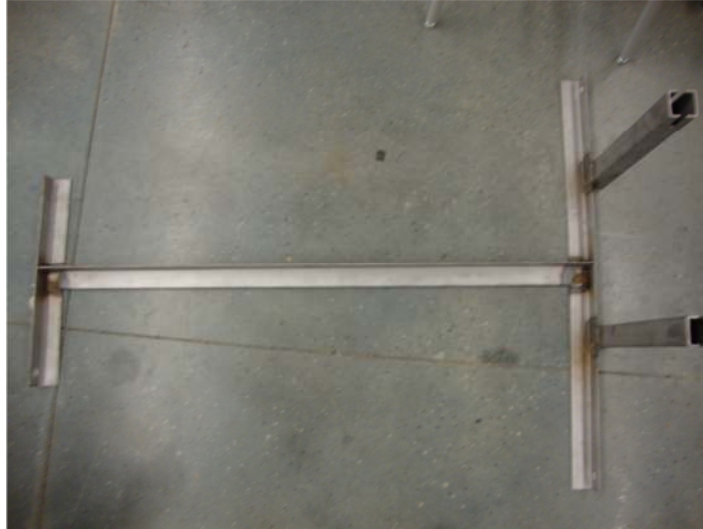
Figure 42: Initial Support Frame
