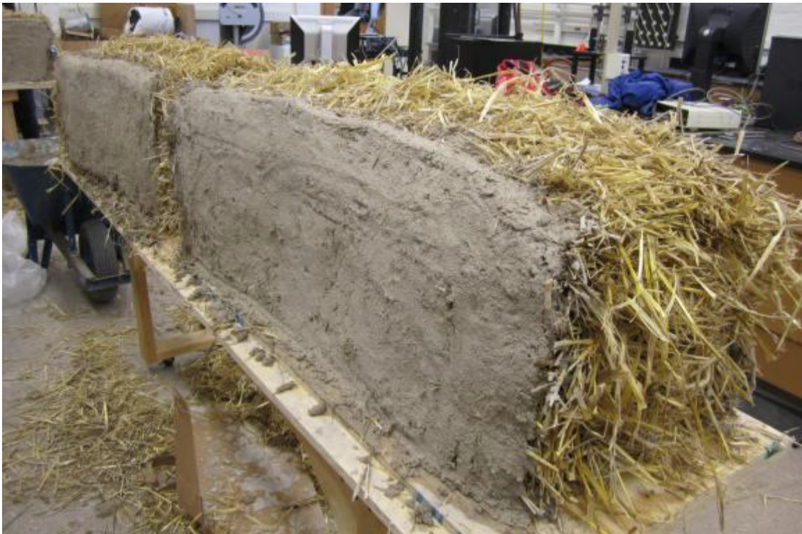
Figure 4 Straw Bale and Plaster Sample
