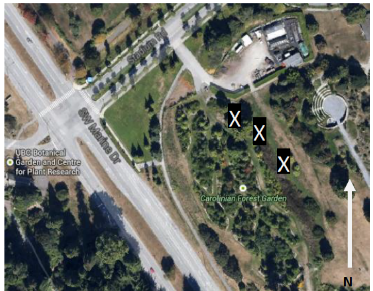
Figure 19 Site Investigation Borehole Locations, denoted by White Xs
