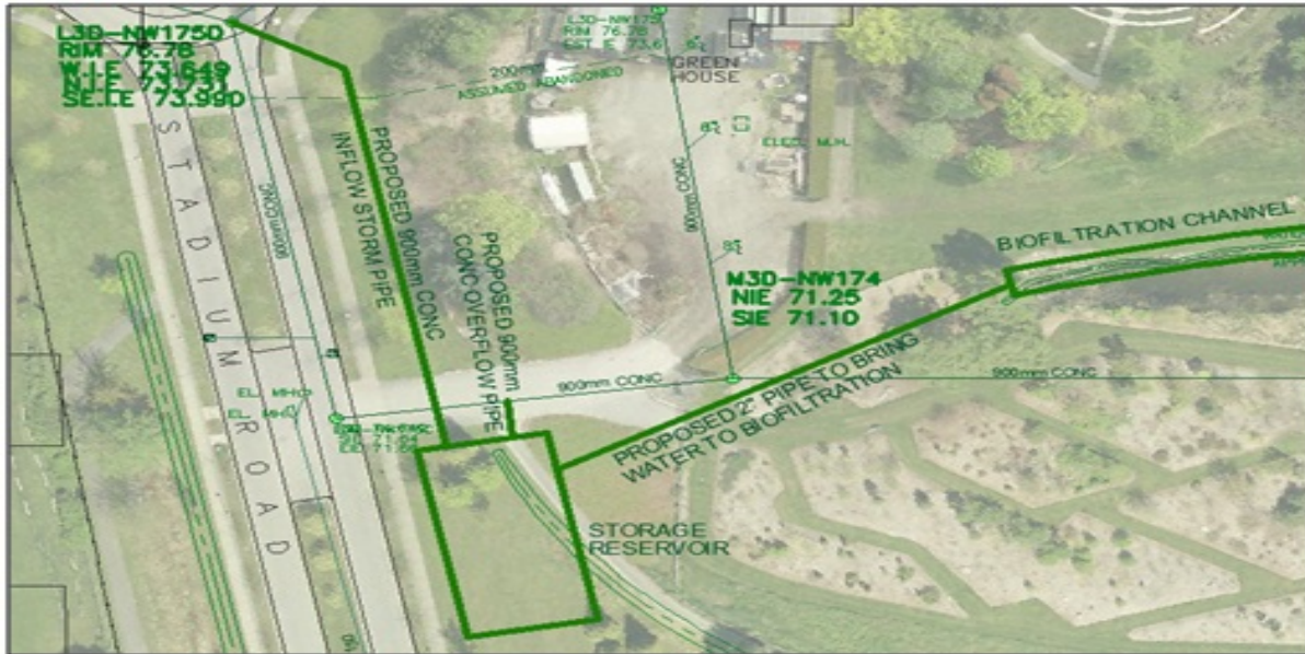
Figure 3 - Location of Collection Pipes
