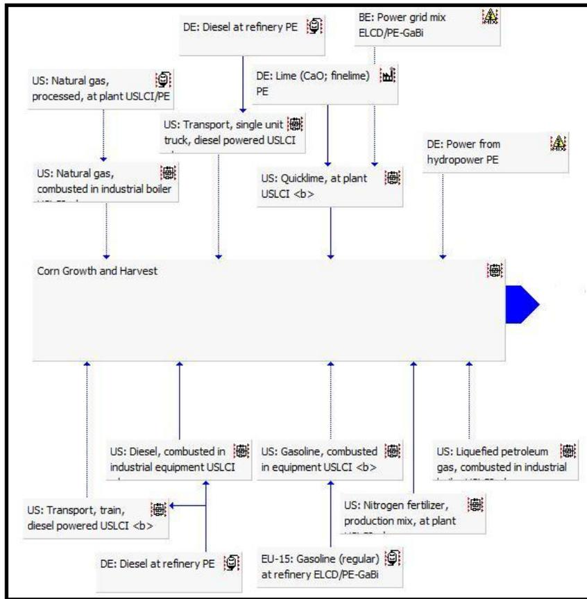
Figure 3.3: Simulation of corn growth and harvesting in GaBi
