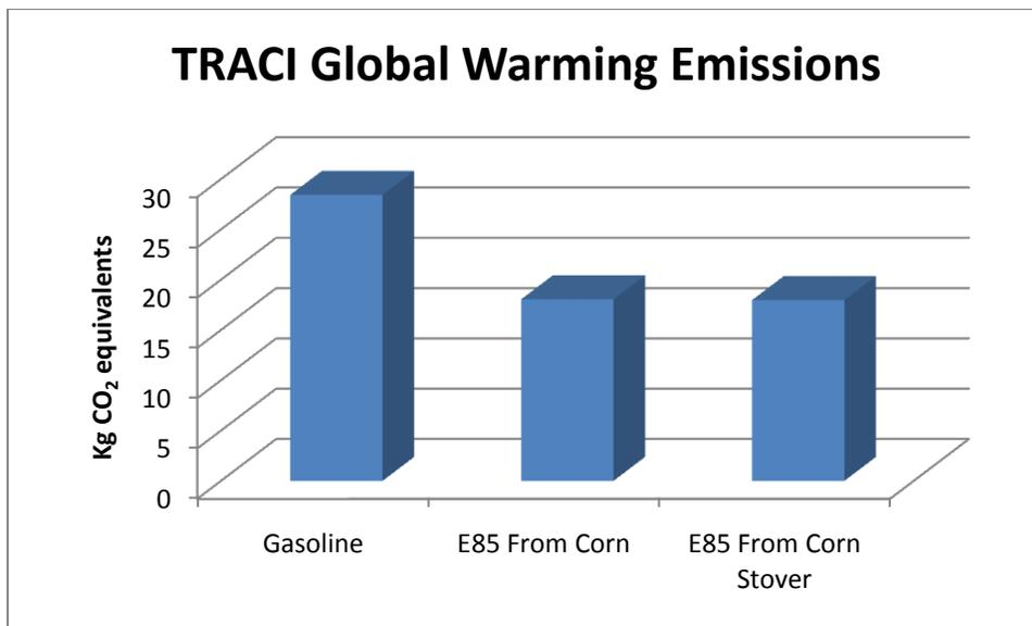
Figure 4.0 Comparison of green house gas emissions for each LCA
