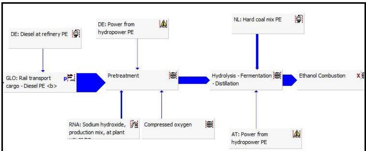
Figure 3.7: Simulation of ethanol production from corn stover in GaBi
