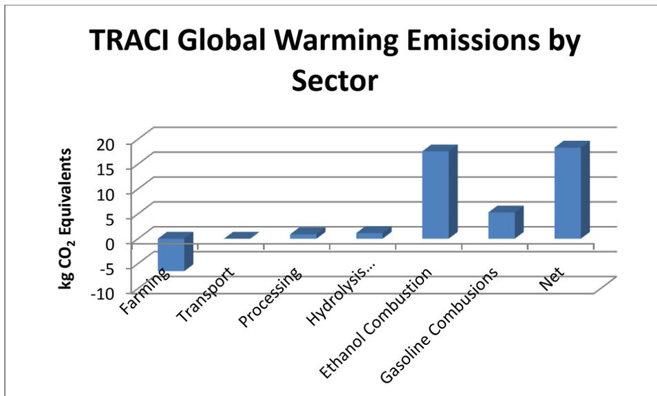
Figure 3.5: Global warming emissions by sector for E85 produced from corn
