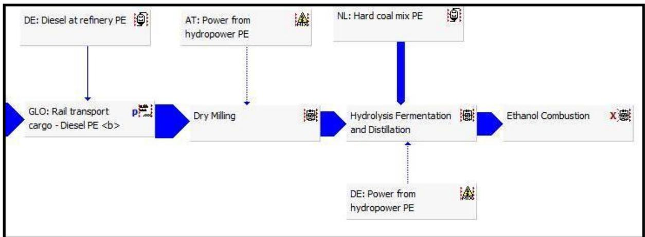
Figure 3.4: Simulation of Ethanol Production from Corn in GaBi
