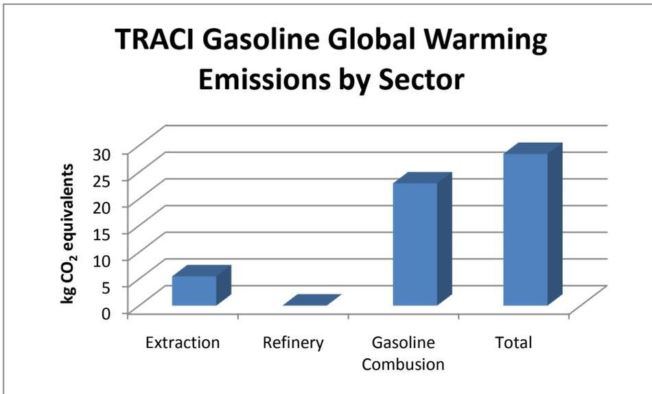
Figure 2.3: Global Warming (CO<sub>2</sub> equivalents) emissions from gasoline LCA based on 100km travelled
