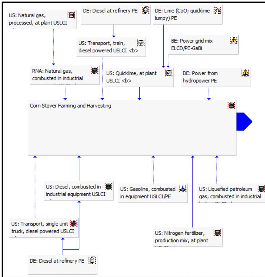
Figure 3.6: Simulation of corn stover growth and harvesting on GaBi
