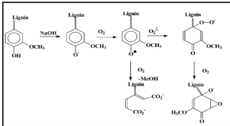
Figure 3.2: Reaction mechanism for oxygen delignification ((Lucia & Smereck, 2001)13)
