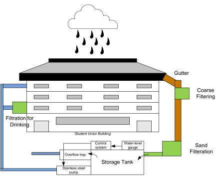
Figure 4: Rainwater harvesting system block diagram
