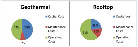
Figure 2: Cost Breakdown of Geothermal and Rooftop HVAC Units
