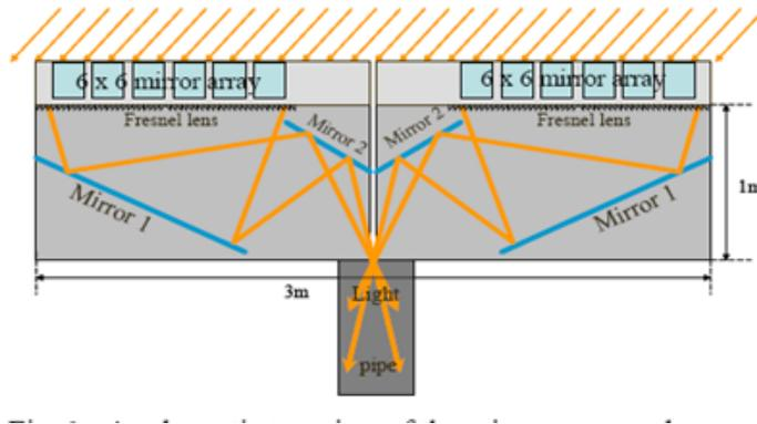
*Figure 1 – A Schematic Top View of the Mirror Array and Redirecting Optics Within the Canopy Structure (1)*
