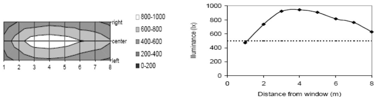
Figure 6 – Luminance Distribution Due to Solar Canopy (1)
