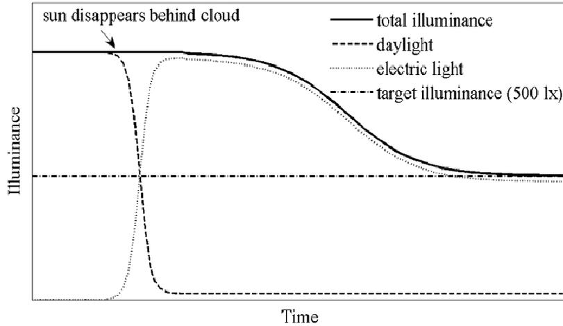
*Figure 8 – Change in the Distribution of Light Sources When the Sun Disappears Behind a Cloud (1)*
