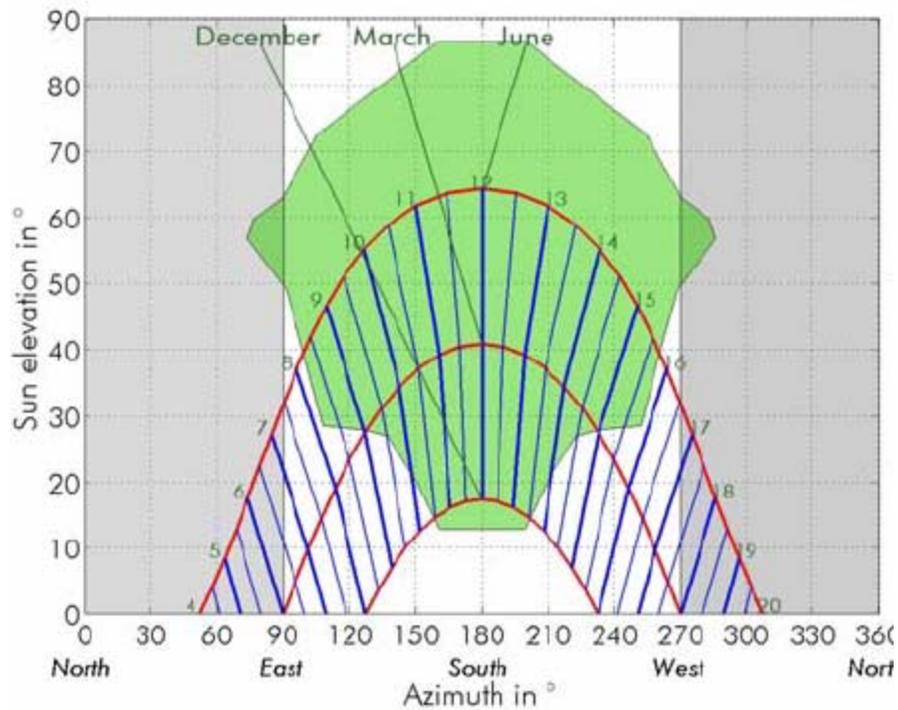
*Figure 9 – Periods During the Year Where Solar Canopy is Sufficient to Provide All Lighting (1)*
