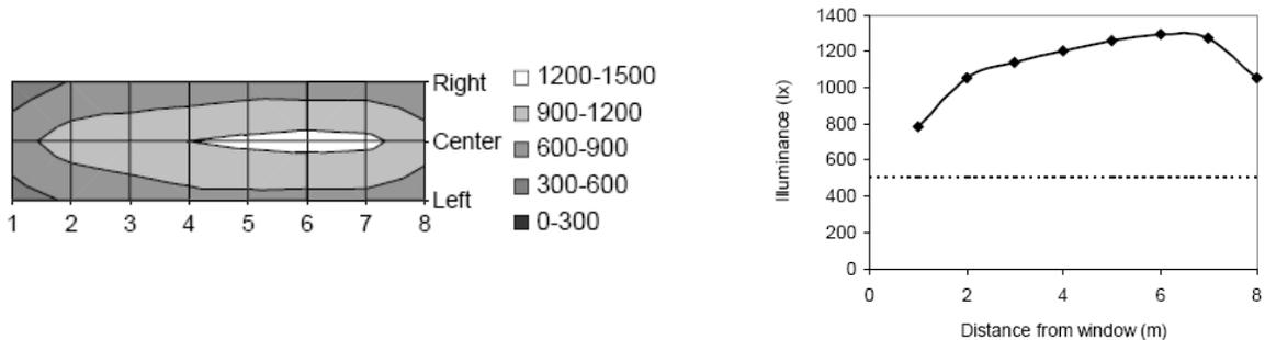
Figure 5 – Luminance Distribution Due to Electrical Lighting (1)
