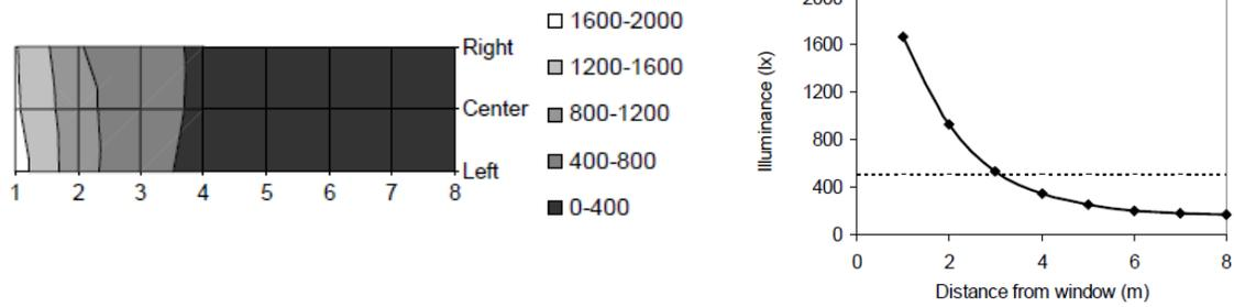
Figure 4 – Luminance Distribution Due to South Wall Window(1)
