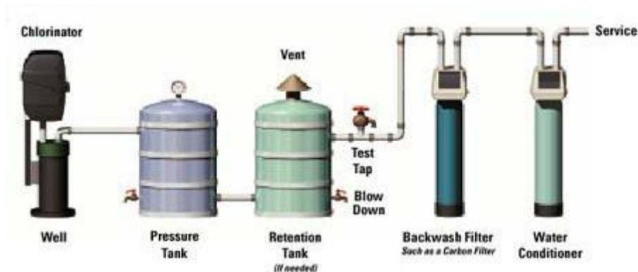
Figure 2 : Pellet Chlorination System(Excel Water Technologies, 2007)
