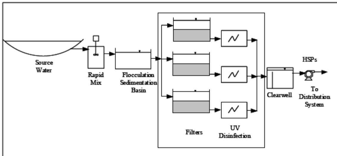
Figure 3 : Schematic of UV disinfection installation upstream of a clearwell (Lehr et al., 2005)
