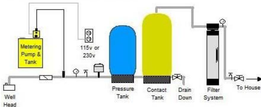
Figure 1 : Chlorine Injection System (Excel Water Technologies, 2007)
