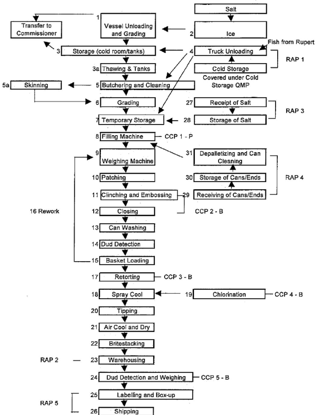
**Fig. 5.** Processing and packaging flow chart of canned fish (D. Safrika, Personal Communications, March 24, 2009).
